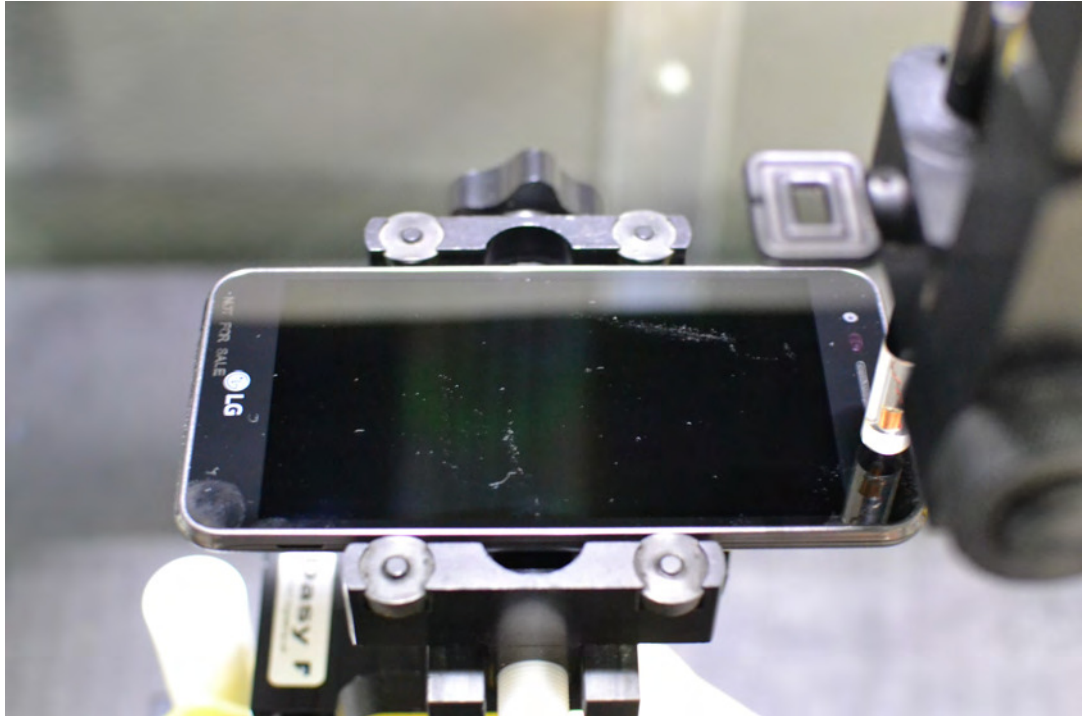
Figure 13-1 Test Setup for Wireless Device
