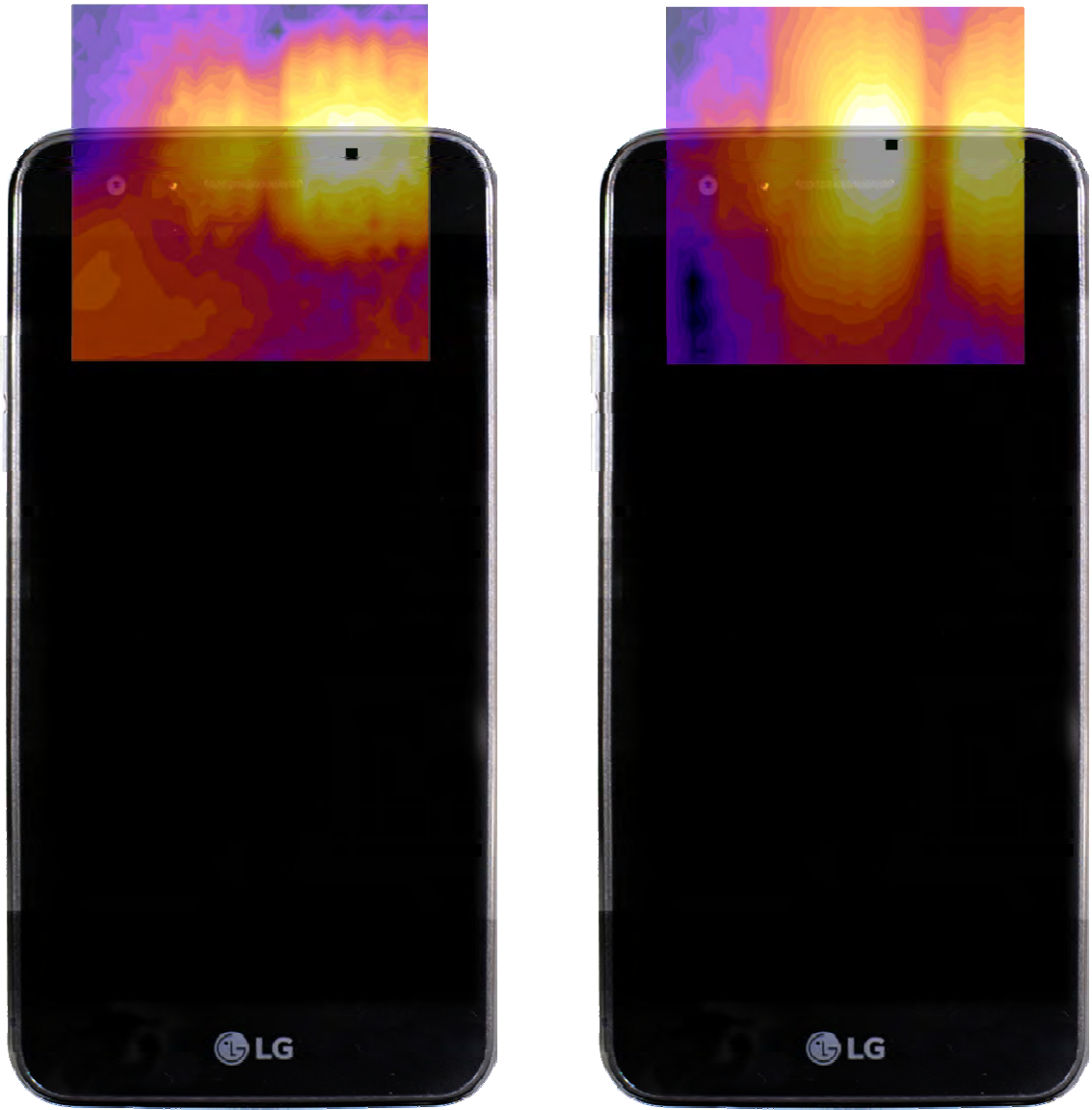
Figure 13-3 T-Coil Scan Overlay Magnetic Field Distributions
