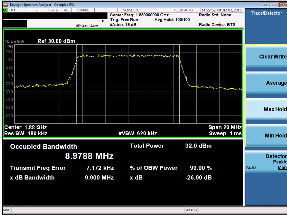
Plot 7-23. Occupied Bandwidth Plot (Band 2 – 10.0MHz QPSK – RB Size 50)
