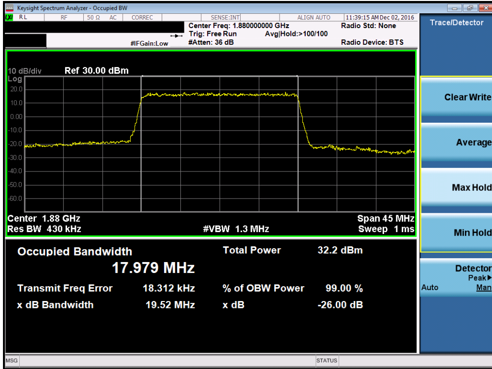
Plot 7-27. Occupied Bandwidth Plot (Band 2 – 20.0MHz QPSK – RB Size 100)
