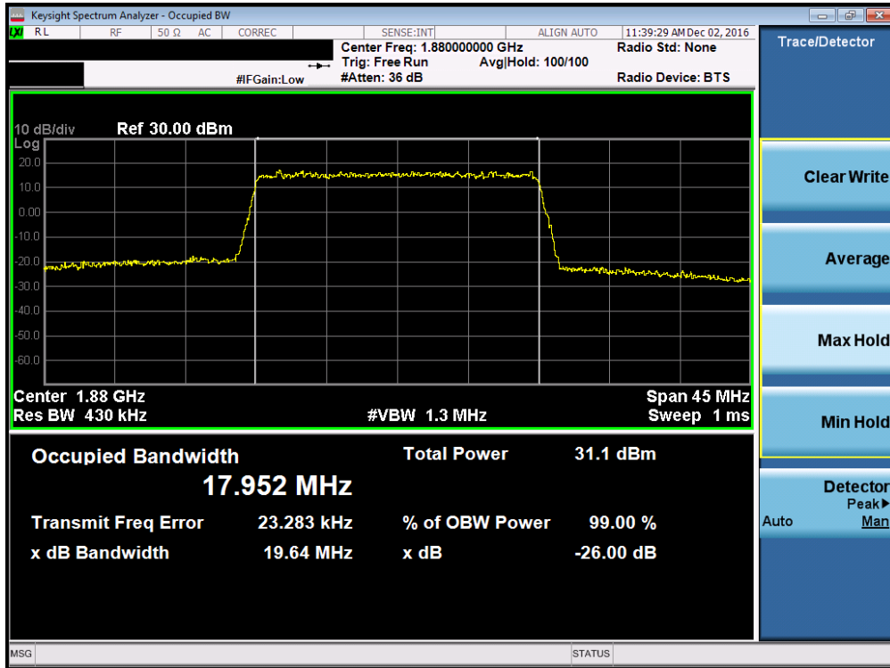
Plot 7-28. Occupied Bandwidth Plot (Band 2 – 20.0MHz 16-QAM – RB Size 100)
