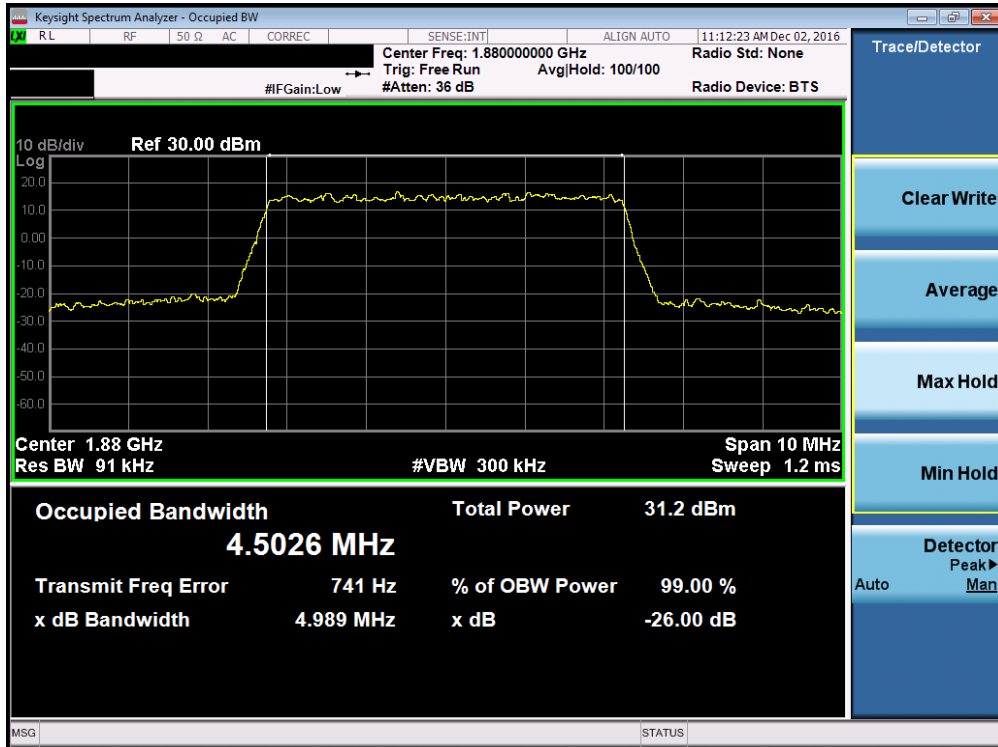
Plot 7-22. Occupied Bandwidth Plot (Band 2 – 5.0MHz 16-QAM – RB Size 25)
