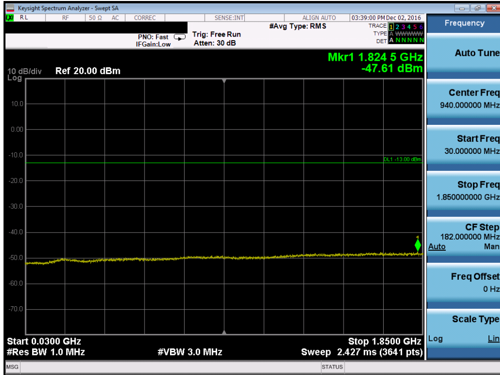
Plot 7-15. Conducted Spurious Plot (PCS CDMA Mode – Ch. 600)
