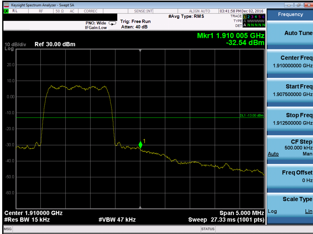
Plot 7-27. Band Edge Plot (PCS CDMA Mode – Ch. 1175)
