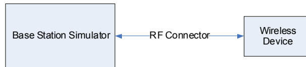
Figure 9-1 Power Measurement Setup
