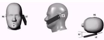
Figure 6-2 Front, Side and Top View of Ear/15º Tilt Position
