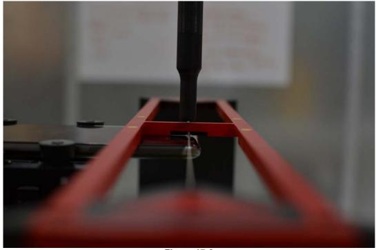
Figure 17-2 **HAC Phantom Plane Alignment**
