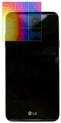
Figure 17-4 E-Field WD Scan overlay (T-coil centered scan area pictured)
