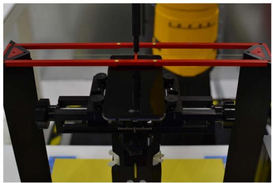
Figure 17-1 Ear Reference Point HAC Phantom Alignment
