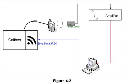
T-Coil Test Setup
