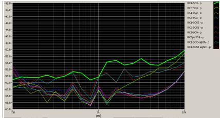
Figure 5-1 CDMA Audio Band Magnetic Noise
