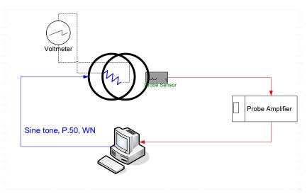
Figure 4-1 Validation Setup with Helmholtz Coil
