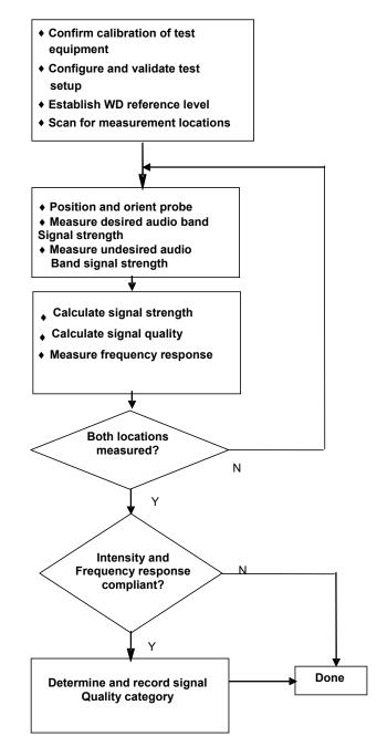
Figure 4-15 C63.19 T-Coil Signal Test Process
