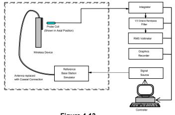
Figure 4-13 Audio Magnetic Field Test Setup
