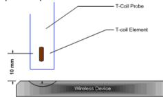
Figure 4-11 **Measurement Distance**
