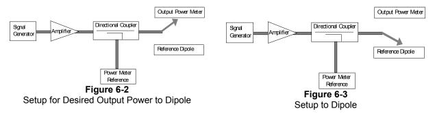
Using this setup configuration, the signal generator was adjusted for the desired output power (100mW) at a specified frequency. The reference power from the coupled port of the directional coupler is recorded. Next, the output cable is connected to the reference dipole, as shown in Figure 6-3.
