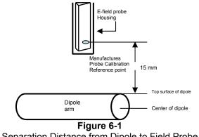
Separation Distance from Dipole to Field Probe
