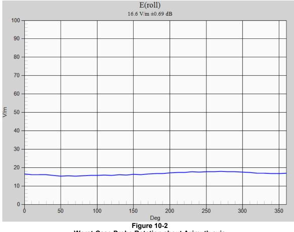
Worst-Case Probe Rotation about Azimuth axis
