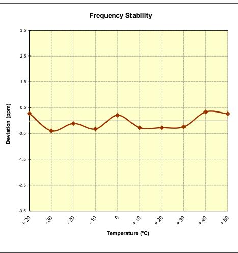
Figure 7-8. Frequency Stability Graph (Band 13)
