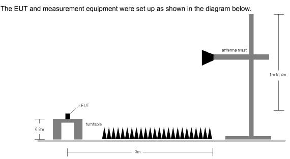
Figure 7-7. Test Instrument & Measurement Setup
