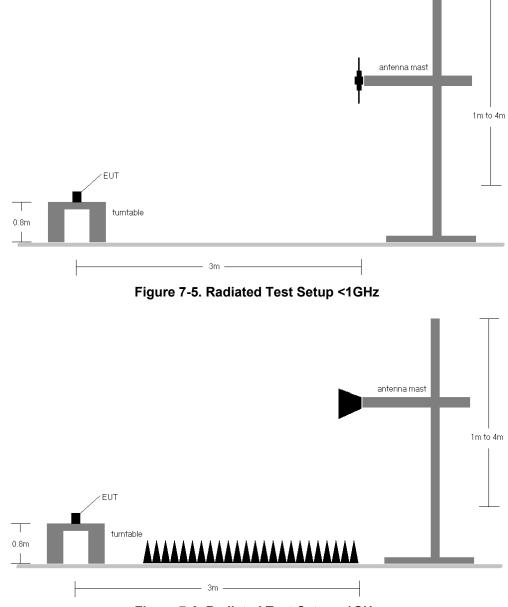
Figure 7-6. Radiated Test Setup >1GHz
