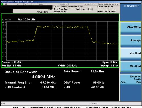
Plot 7-21. Occupied Bandwidth Plot (Band 2 – 5.0MHz QPSK – RB Size 25)
