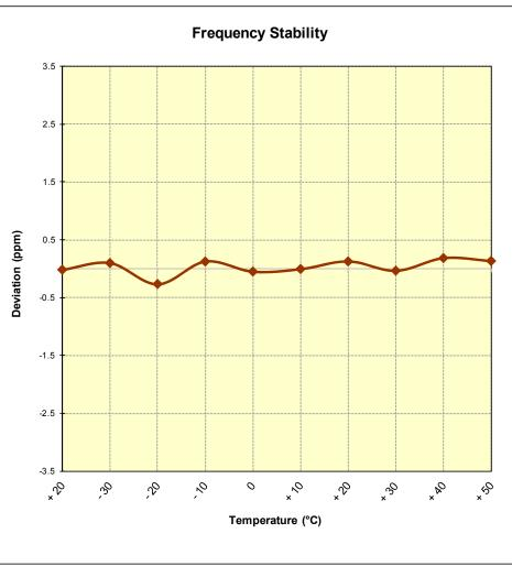
Figure 7-9. Frequency Stability Graph (Band 4)
