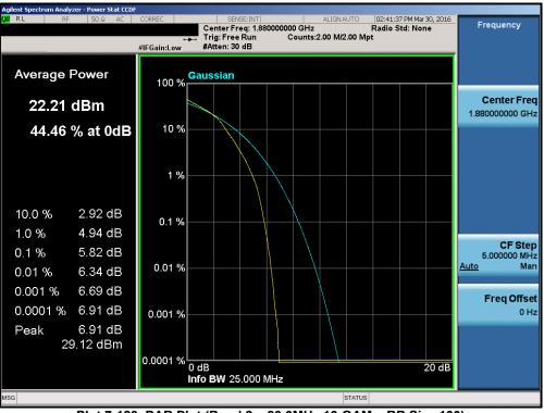
Plot 7-123. PAR Plot (Band 2 – 20.0MHz 16-QAM – RB Size 100)
