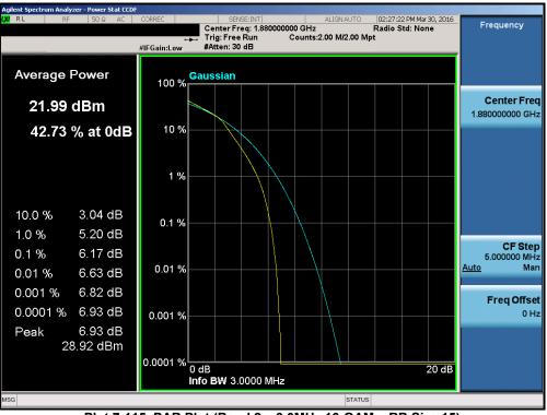
Plot 7-115. PAR Plot (Band 2 – 3.0MHz 16-QAM – RB Size 15)
