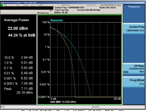
Plot 7-119. PAR Plot (Band 2 - 10.0MHz 16-QAM - RB Size 50)
