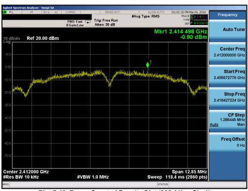
Plot 7-10. Power Spectral Density Plot (802.11b - Ch. 1)
