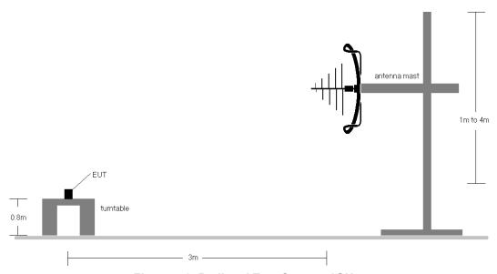
Figure 7-8. Radiated Test Setup < 1GHz
