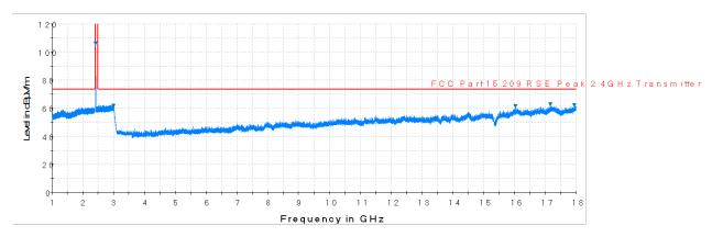
Plot 7-36. Radiated Spurious Plot above 1GHz (802.11b - Ch. 1, Ant. Pol. V)
