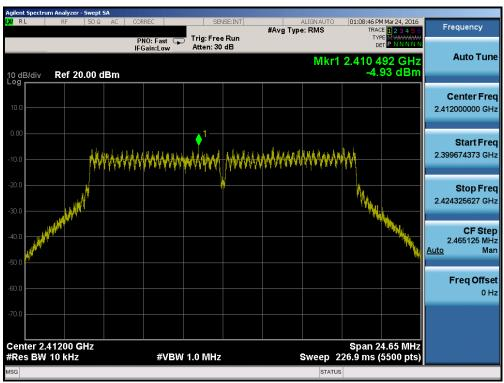
Plot 7-13. Power Spectral Density Plot (802.11g - Ch. 1)
