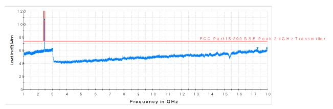
Plot 7-38. Radiated Spurious Plot above 1GHz (802.11b - Ch. 6, Ant. Pol. V)
