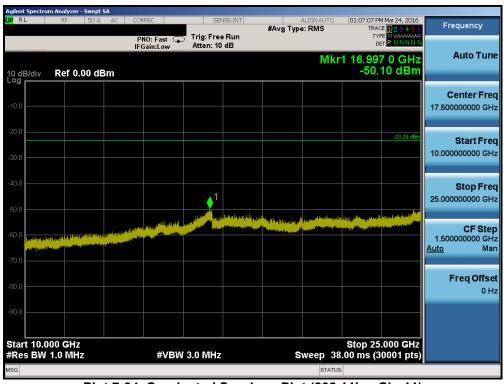
Plot 7-34. Conducted Spurious Plot (802.11b - Ch. 11)
