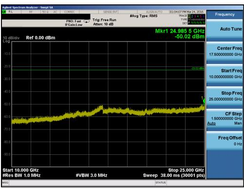
Plot 7-32. Conducted Spurious Plot (802.11b - Ch. 6)
