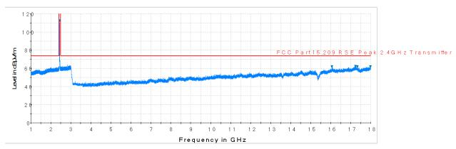
Plot 7-37. Radiated Spurious Plot above 1GHz (802.11b - Ch. 6, Ant. Pol. H)
