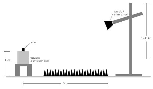
Figure 7-6. Test Instrument & Measurement Setup
