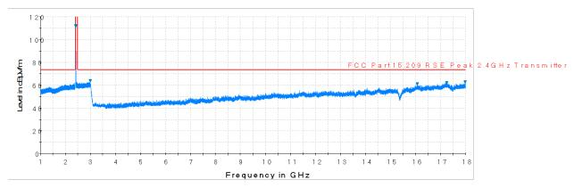
Plot 7-35. Radiated Spurious Plot above 1GHz (802.11b - Ch. 1, Ant. Pol. H)
