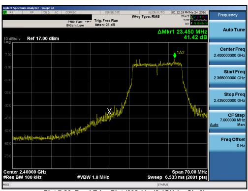
Plot 7-26. Band Edge Plot (802.11n (2.4GHz) - Ch. 2)
