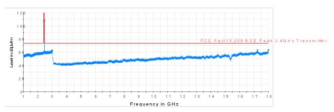
Plot 7-40. Radiated Spurious Plot above 1GHz (802.11b - Ch. 11, Ant. Pol. V)
