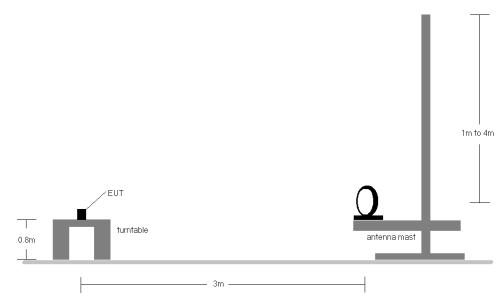
Figure 7-7. Radiated Test Setup < 30Mhz
