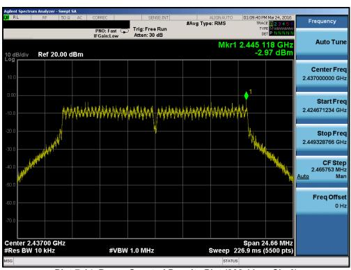
Plot 7-14. Power Spectral Density Plot (802.11g - Ch. 6)
