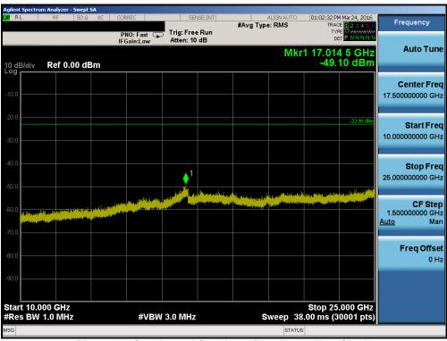
Plot 7-30. Conducted Spurious Plot (802.11b - Ch. 1)
