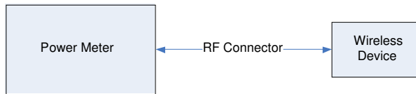
Figure 12-1 Power Measurement Setup
