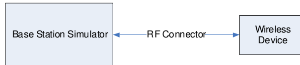
Figure 11-1 Power Measurement Setup
