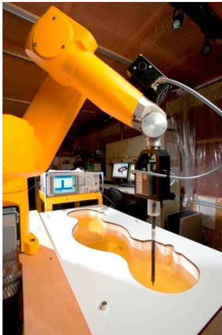
Figure 3-2 SAR Measurement System
