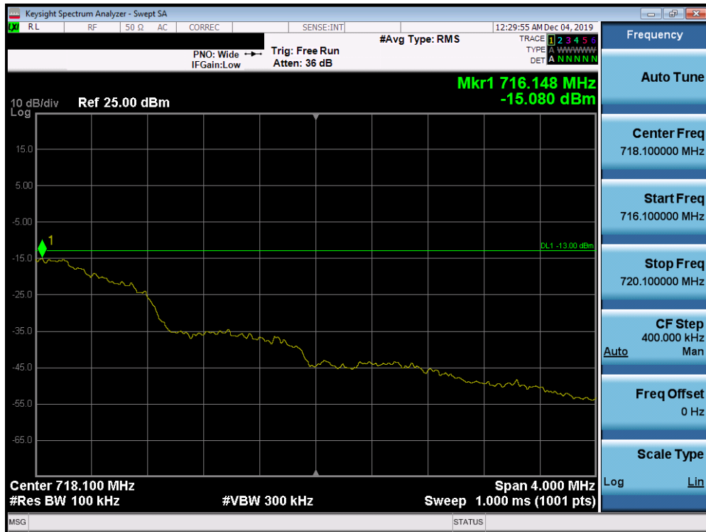
Plot 7-182. Upper Extended Band Edge Plot (Band 12 - 1.4MHz QPSK - Full RB Configuration)
