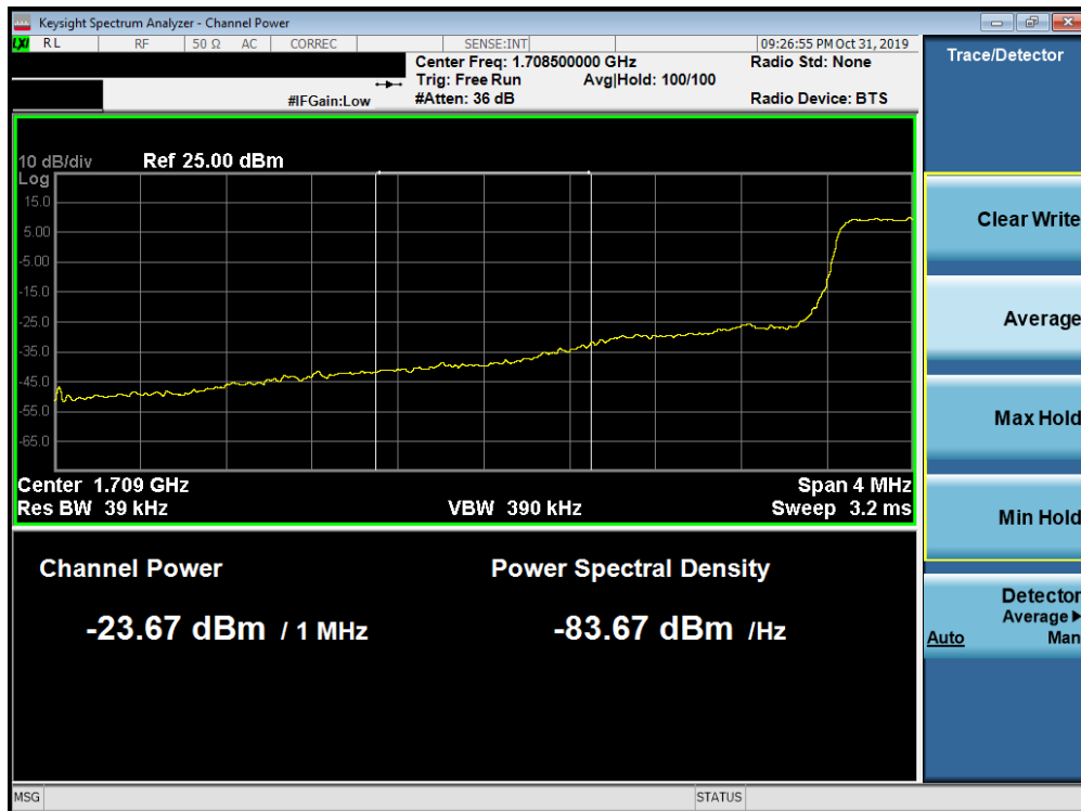
Plot 7-208. Lower Extended Band Edge Plot (Band 66/4 - 1.4MHz QPSK - Full RB Configuration)
