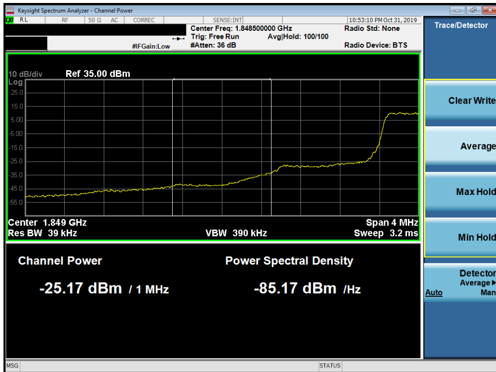
Plot 7-244. Lower Extended Band Edge Plot (Band 25/2 - 1.4MHz QPSK - Full RB Configuration)
