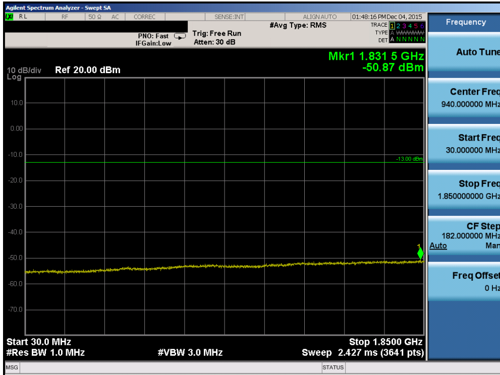
Plot 7-54. Conducted Spurious Plot (Band 2 – 20.0MHz QPSK – RB Size 1, RB Offset 0 – High Channel)
