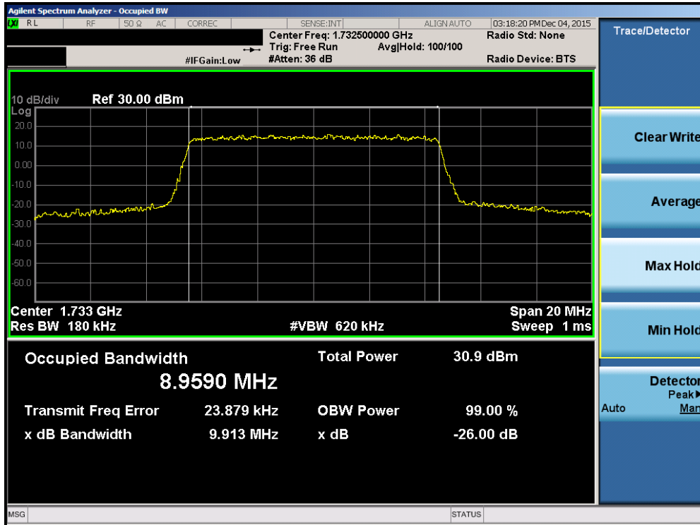
Plot 7-11. Occupied Bandwidth Plot (Band 4 – 10.0MHz QPSK – RB Size 50)
