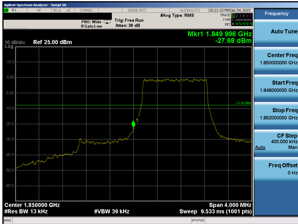
Plot 7-89. Lower Band Edge Plot (Band 2 – 1.4MHz QPSK – RB Size 6)
