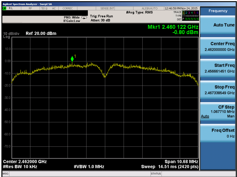
Plot 7-12. Power Spectral Density Plot (802.11b – Ch. 11)
