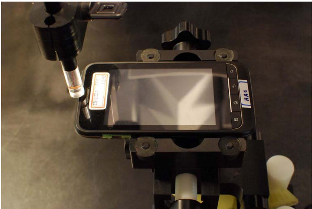
Figure 13-1 Test Setup for Wireless Device
