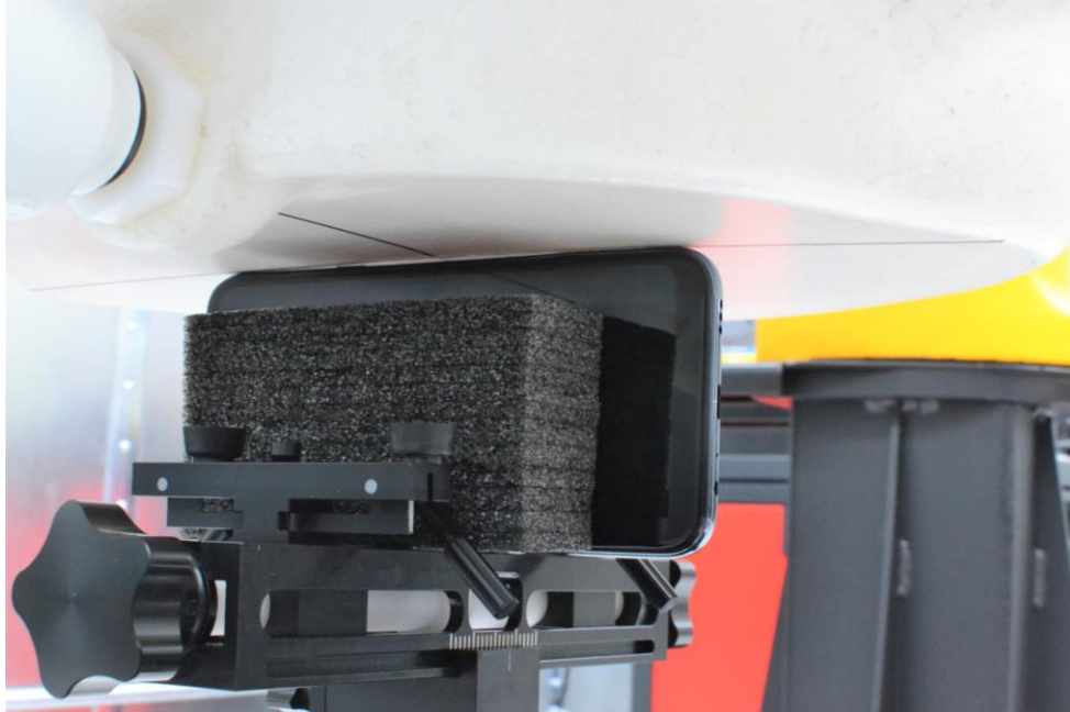
SAR Test Setup Photo 15 – Right Edge at 0 mm
