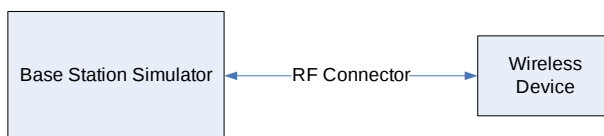
Figure 9-2 Power Measurement Setup
