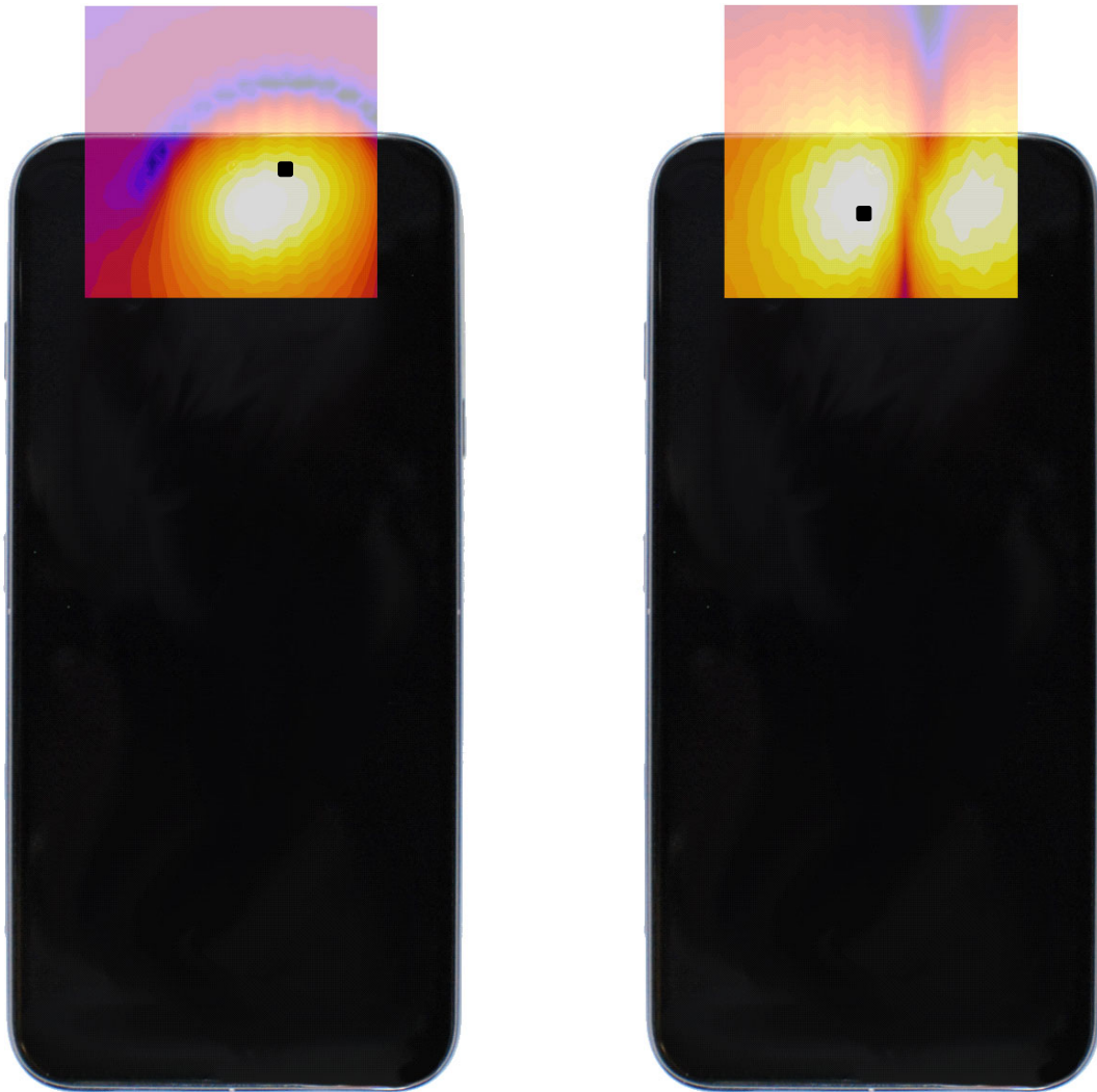
Figure 16-3 T-Coil Scan Overlay Magnetic Field Distributions
