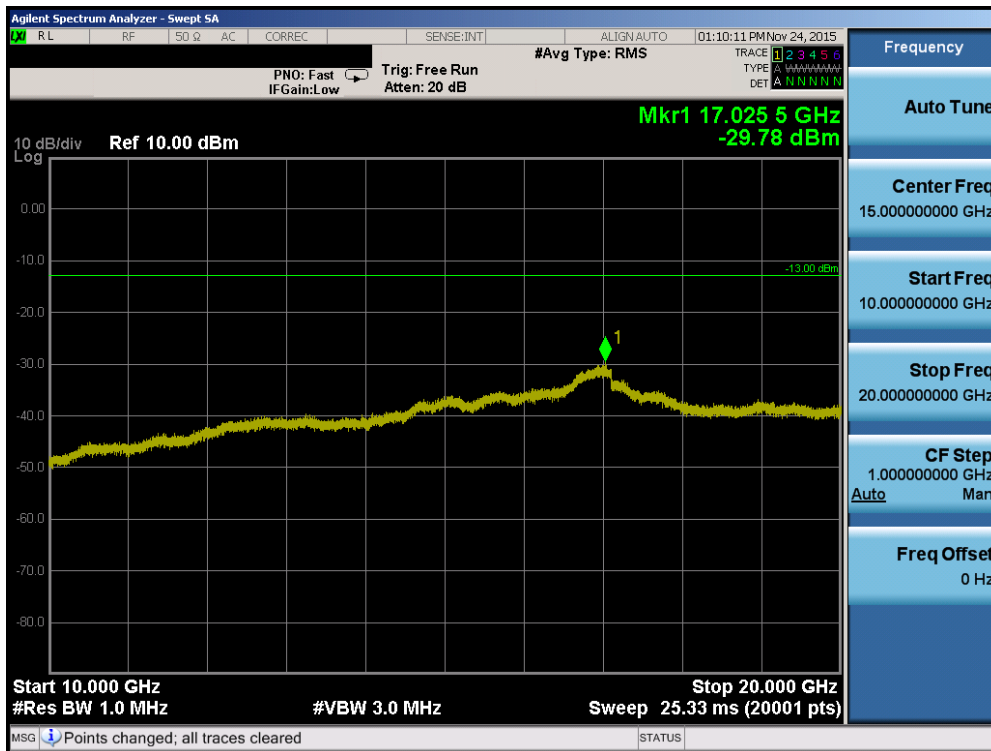
Plot 7-37. Conducted Spurious Plot (AWS WCDMA Mode – Ch. 1312)
