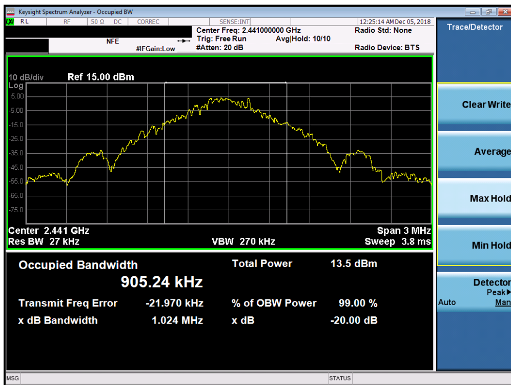
Plot 7-2. 20dB Bandwidth Plot (Bluetooth, 1Mbps – Ch. 39)
