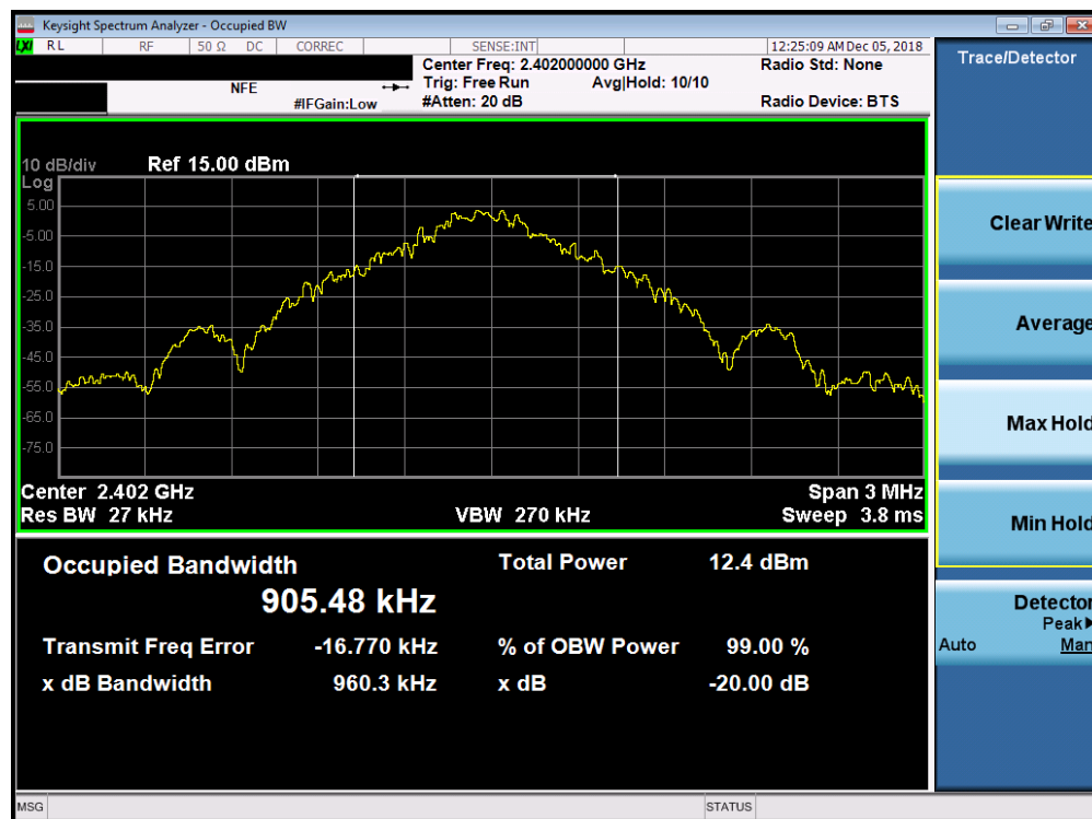
Plot 7-1. 20dB Bandwidth Plot (Bluetooth, 1Mbps – Ch. 0)
