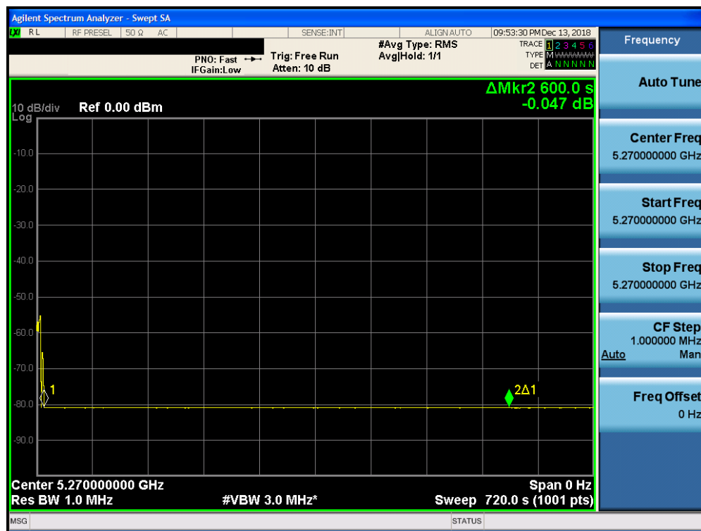
Figure 5-5. Band 2A Client Beacon Test – Monitoring live spectrum – Elapse time 10 minutes
