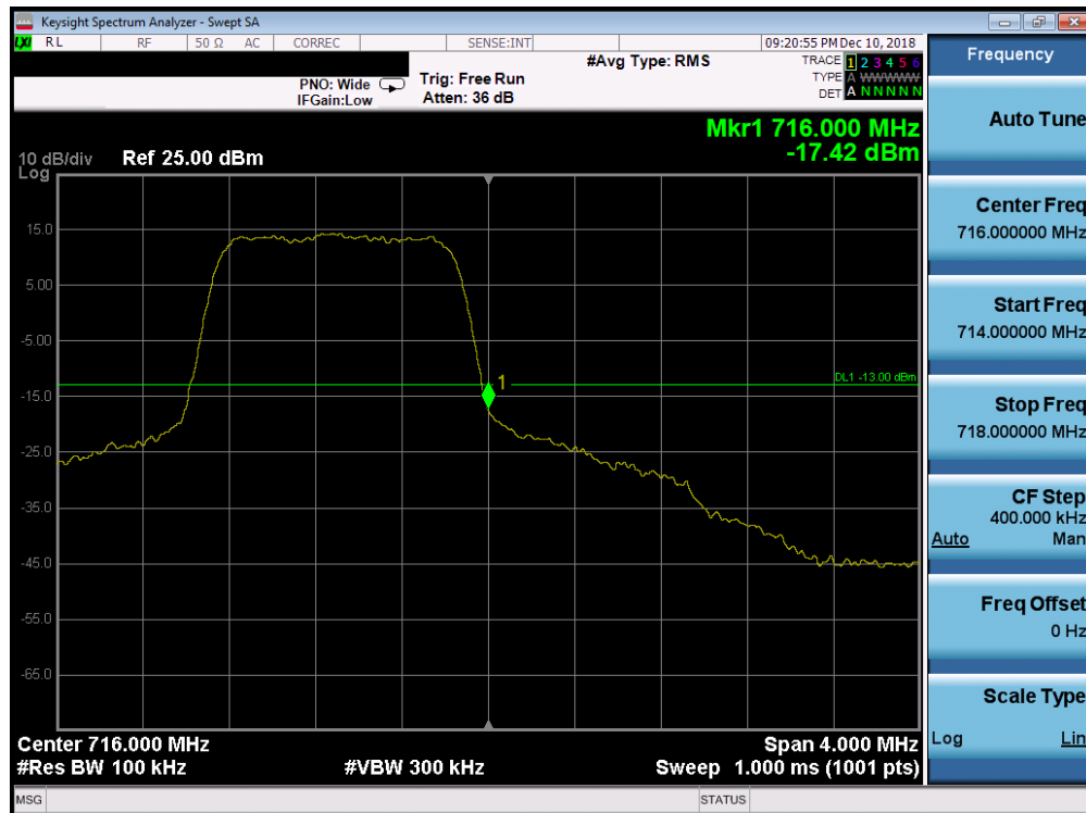
Plot 7-136. Upper Band Edge Plot (Band 12 - 1.4MHz QPSK - Full RB Configuration)
