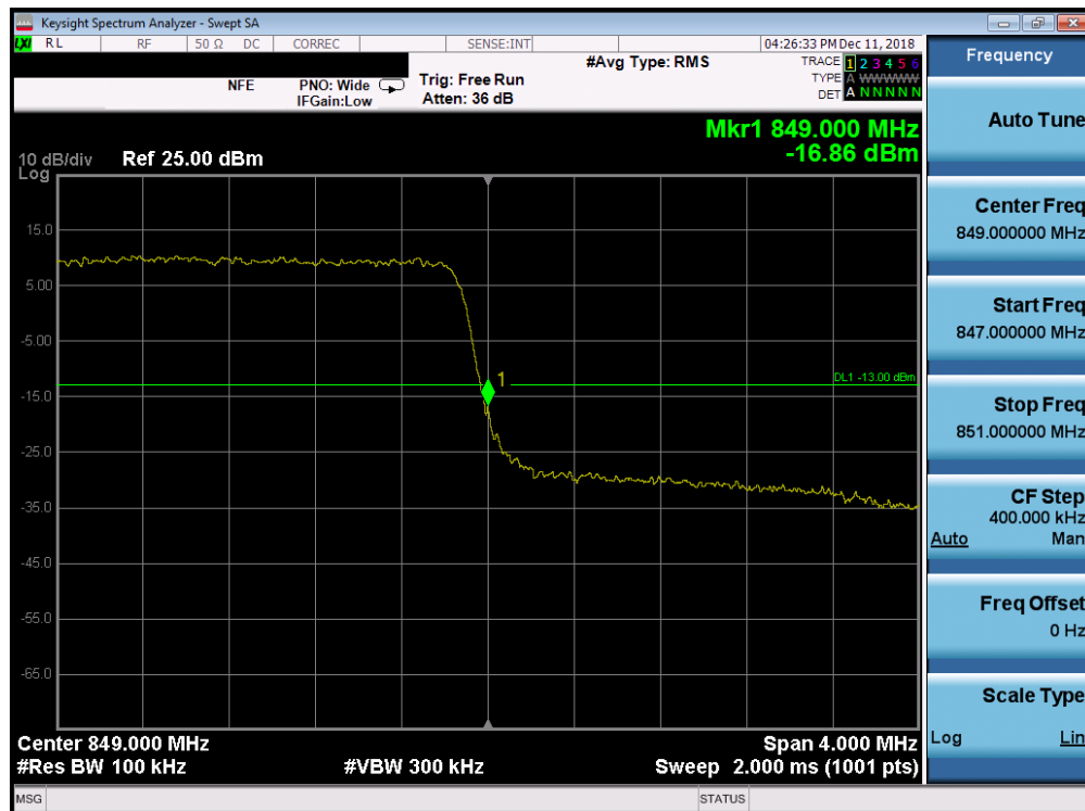
Plot 7-153. Upper Band Edge Plot (Band 5 - 3.0MHz QPSK - Full RB Configuration)
