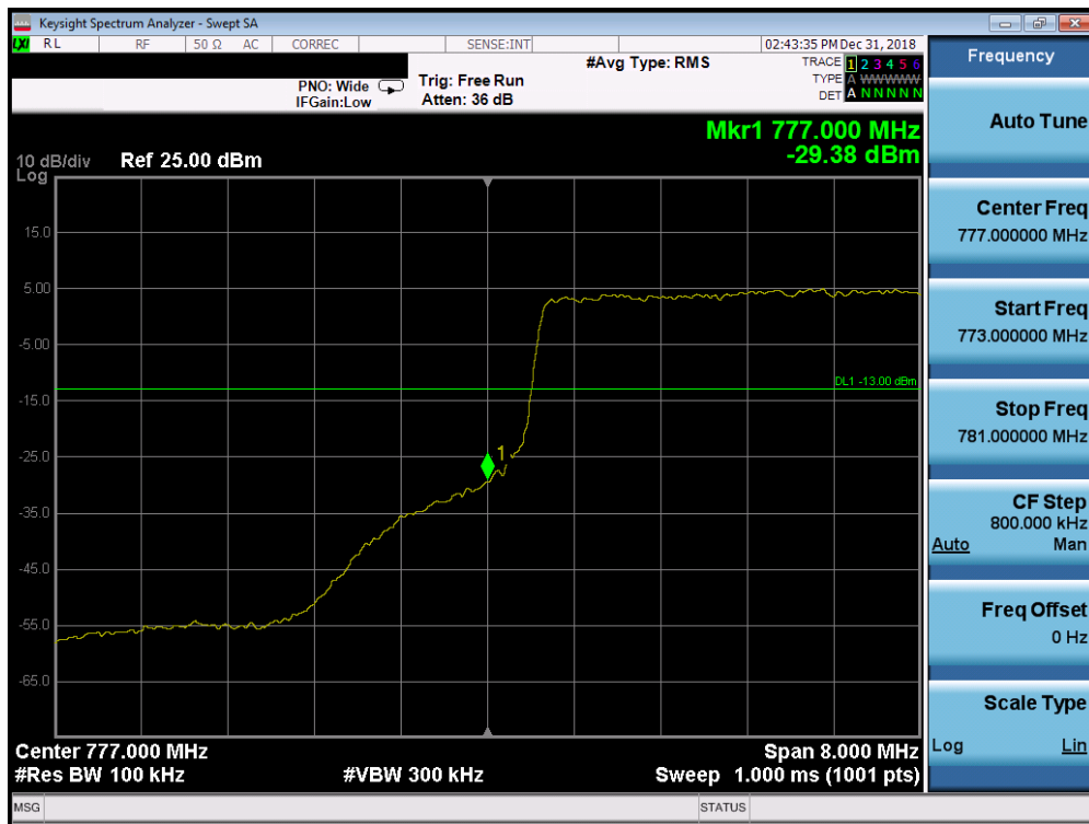
Plot 7-146. Lower Band Edge Plot (Band 13 - 10.0MHz QPSK - Full RB Configuration)
