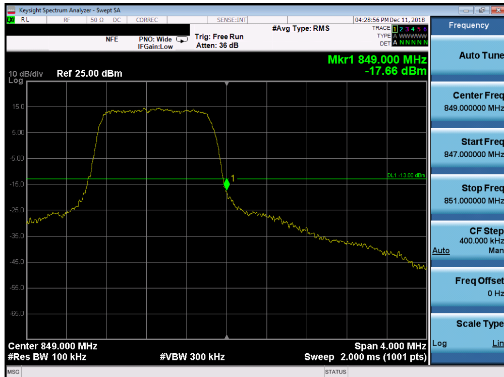
Plot 7-151. Upper Band Edge Plot (Band 5 - 1.4MHz QPSK - Full RB Configuration)
