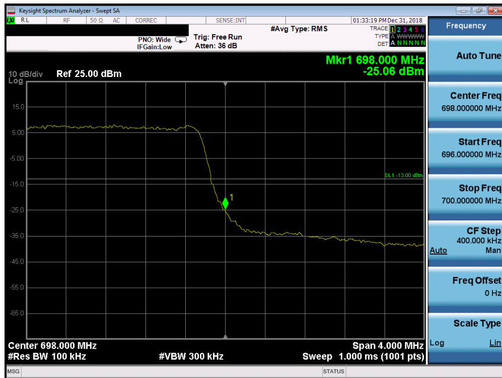
Plot 7-128. Upper Band Edge Plot (Band 71 - 5.0MHz QPSK - Full RB Configuration)
