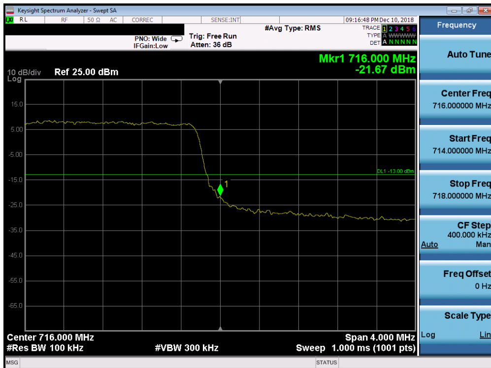
Plot 7-140. Upper Band Edge Plot (Band 12 - 5.0MHz QPSK - Full RB Configuration)
