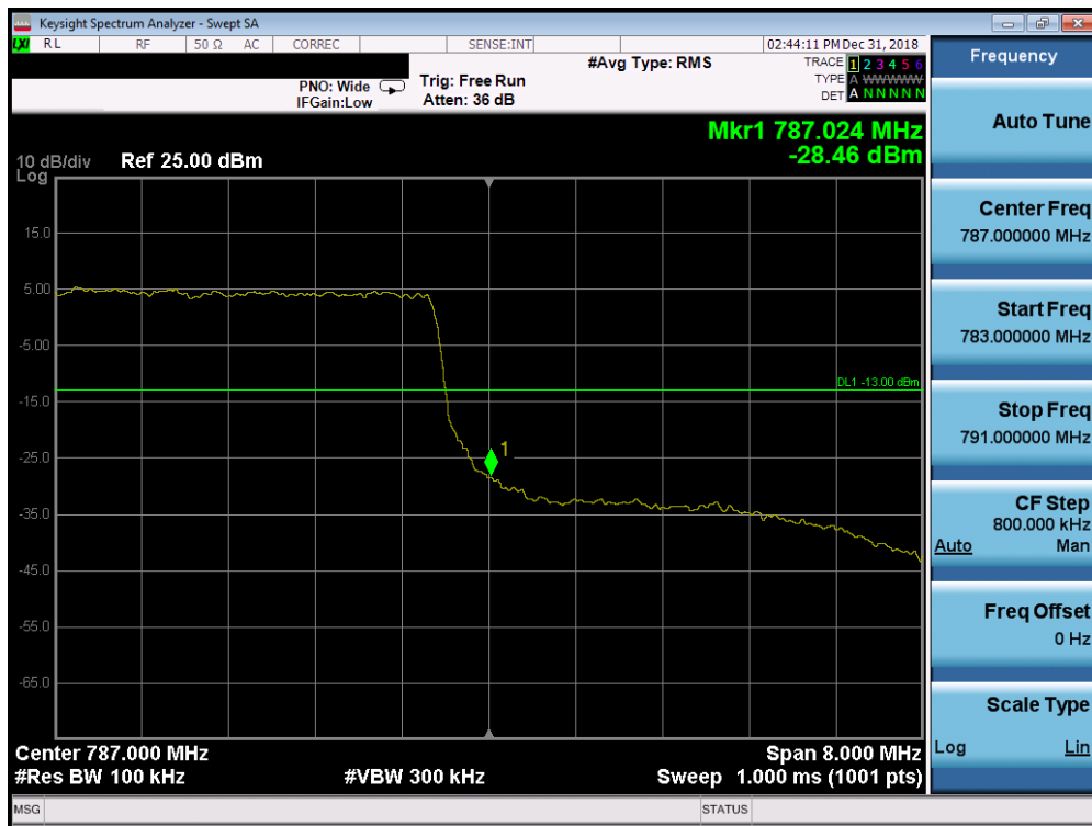
Plot 7-148. Upper Band Edge Plot (Band 13 - 10.0MHz QPSK - Full RB Configuration)
