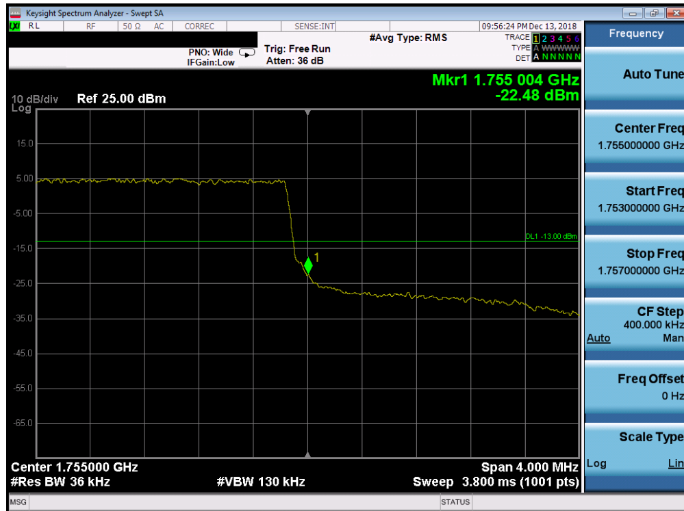
Plot 7-166. Upper Band Edge Plot (Band 4 - 3.0MHz QPSK - Full RB Configuration)
