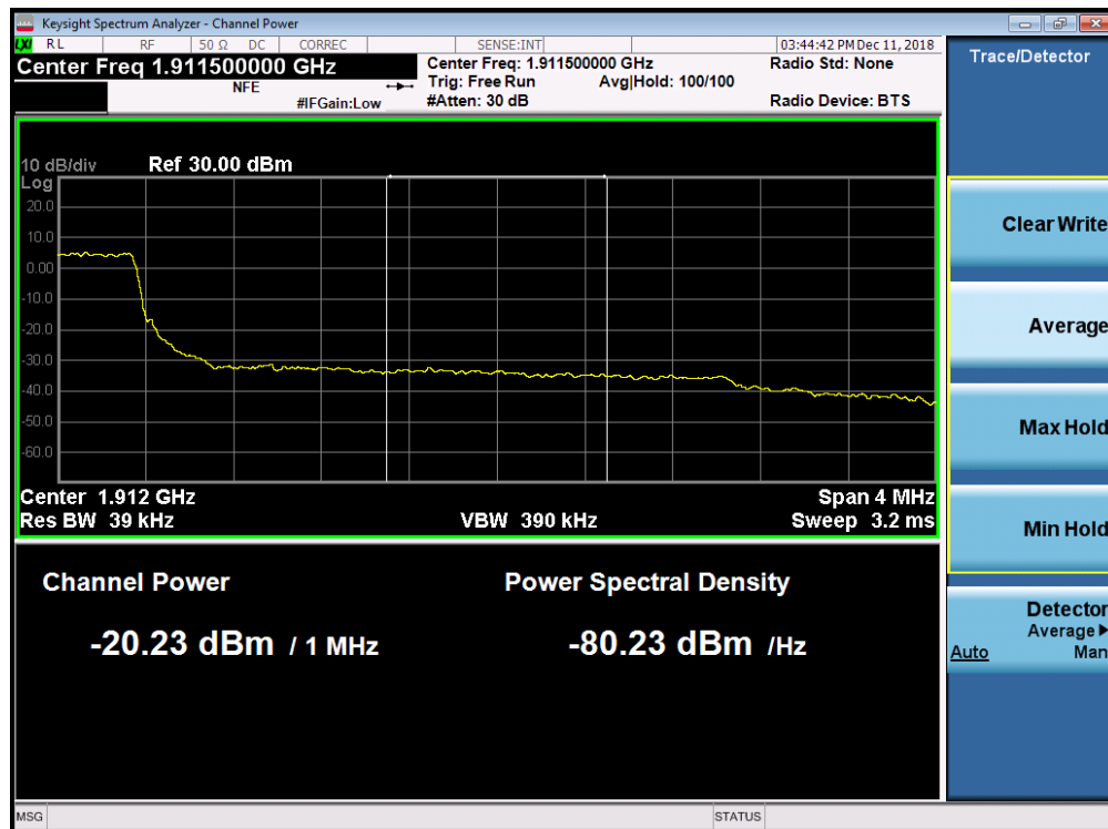
Plot 7-201. Upper Extended Band Edge Plot (Band 2 - 3.0MHz QPSK - Full RB Configuration)
