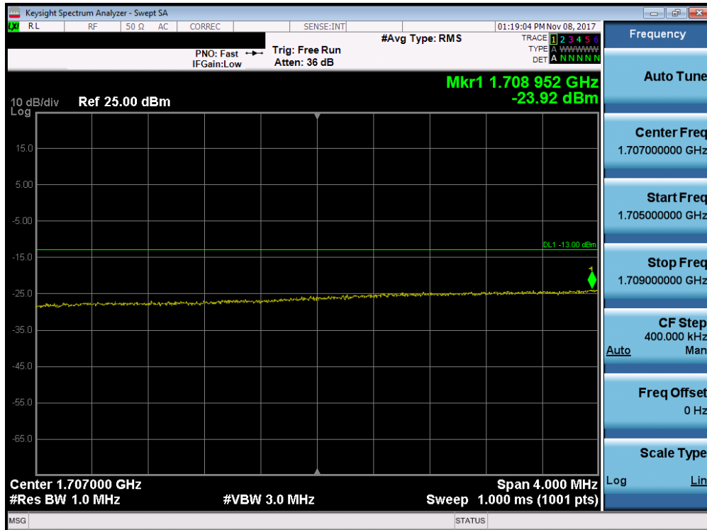
Plot 7-130. . Lower Extended Band Edge Plot (Band 66 - 15.0MHz QPSK - Full RB Configuration)
