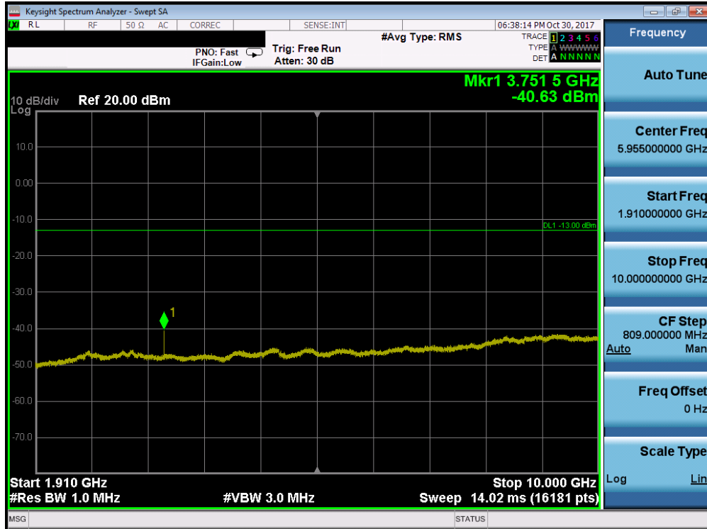
Plot 7-78. Conducted Spurious Plot (Band 2 - 10.0MHz QPSK - RB Size 1, RB Offset 0 - Mid Channel)
