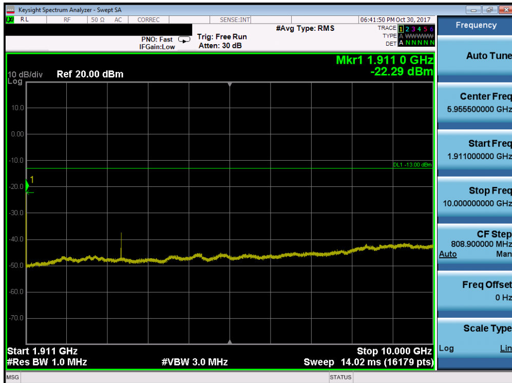
Plot 7-81. Conducted Spurious Plot (Band 2 - 10.0MHz QPSK - RB Size 1, RB Offset 0 - High Channel)
