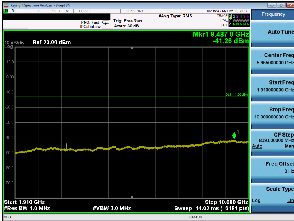
Plot 7-75. Conducted Spurious Plot (Band 2 - 10.0MHz QPSK - RB Size 1, RB Offset 0 - Low Channel)
