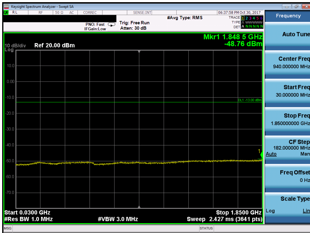
Plot 7-77. Conducted Spurious Plot (Band 2 - 10.0MHz QPSK - RB Size 1, RB Offset 0 - Mid Channel)
