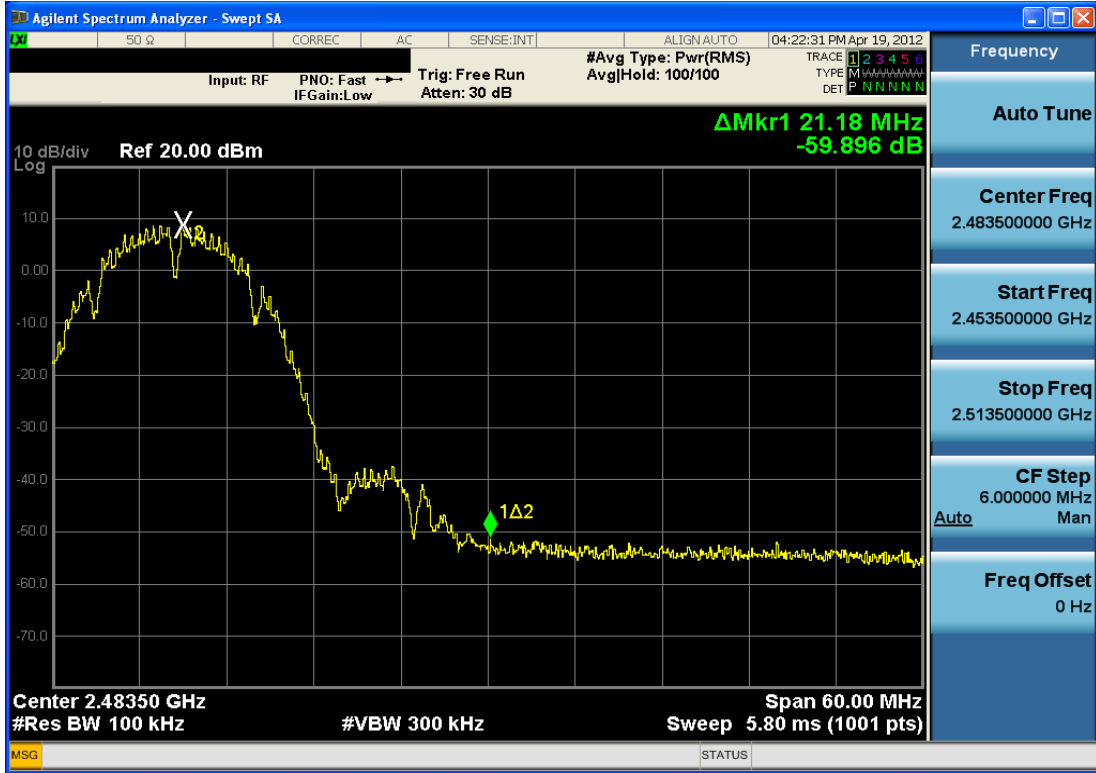
Plot 6-20. Band Edge Plot (802.11b – Ch. 11)
