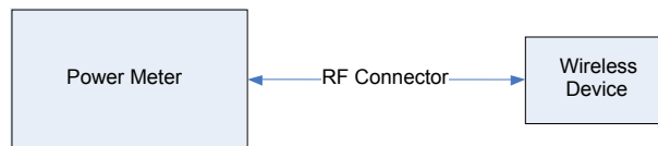
Figure 9-3 Power Measurement Setup
