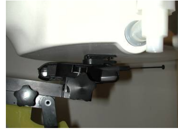
Figure 6-4 Body SAR Sample Photo (Not Actual EUT)
