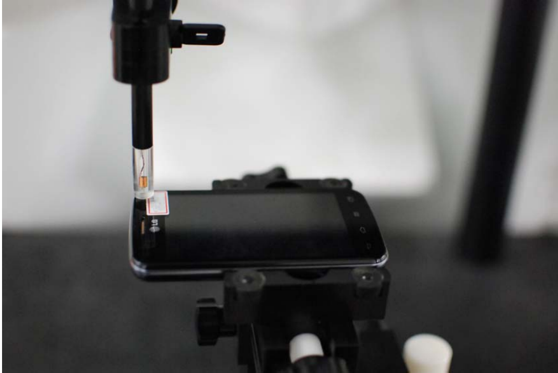
Figure 13-1 Test Setup for Wireless Device
