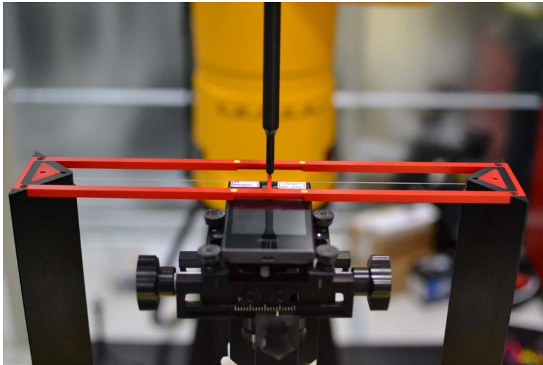
Figure 17-1 Ear Reference Point HAC Phantom Alignment
