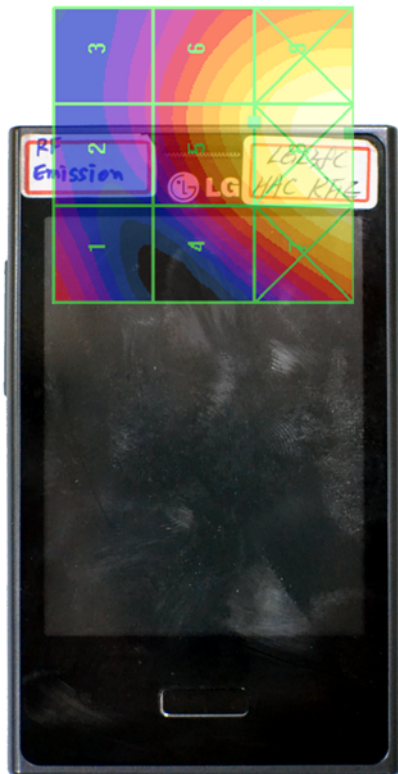
Figure 17-4 E-Field WD Scan overlay
