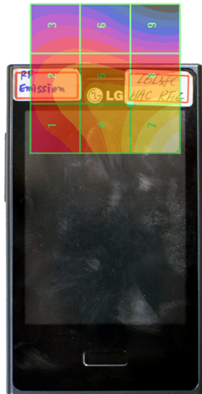
Figure 17-5 H-Field WD Scan overlay
