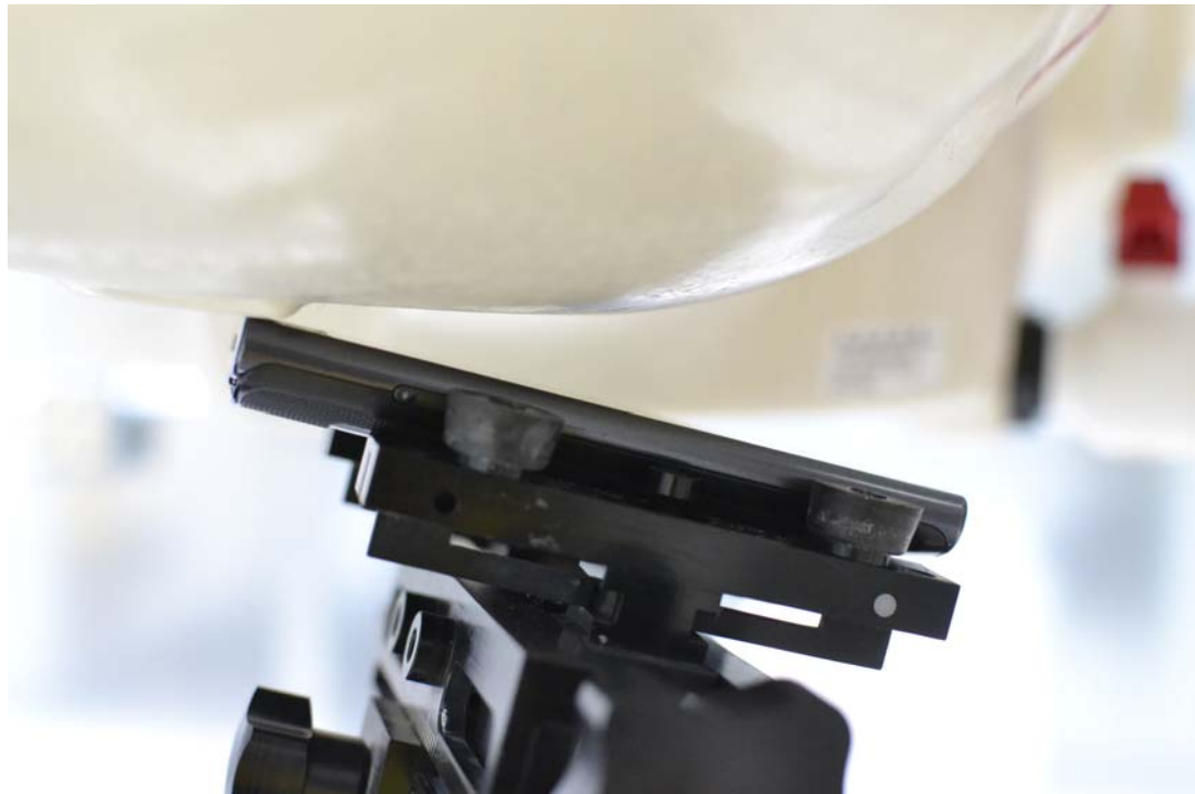
SAR Test Setup Photo 2 - Right Tilt
