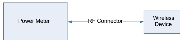
Figure 9-2 Power Measurement Setup
