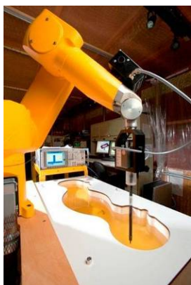
Figure 3-1 SAR Measurement System
