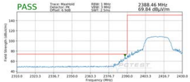
Plot 7-40. Radiated Restricted Lower Band Edge Measurement (Peak)
