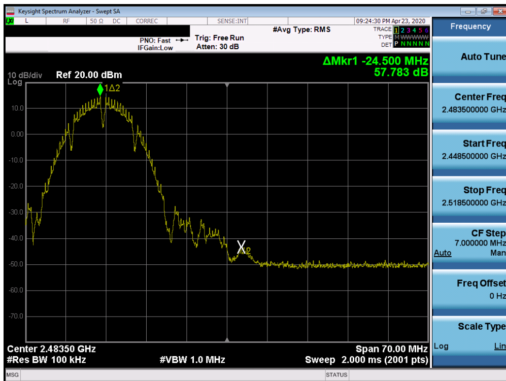
Plot 7-20. Band Edge Plot (802.11b – Ch. 11)
