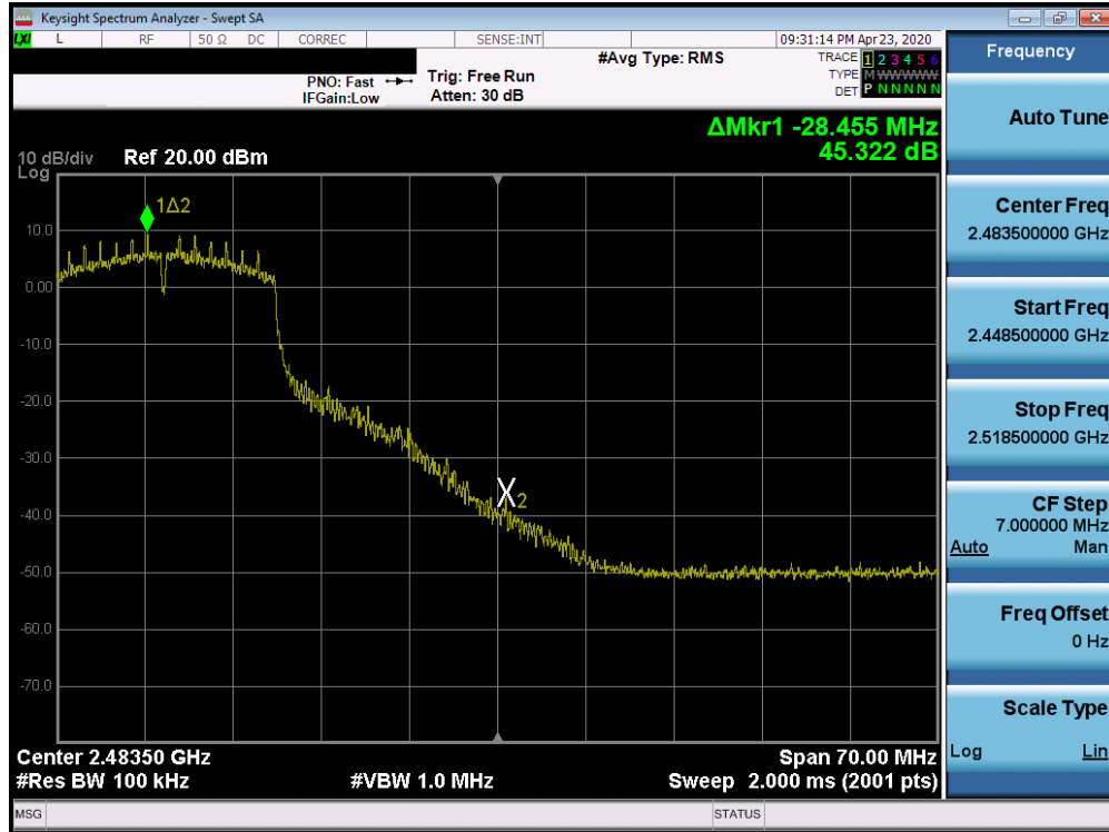
Plot 7-27. Band Edge Plot (802.11n (2.4GHz) – Ch. 10)
