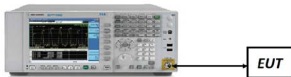
Figure 7-2. Test Instrument & Measurement Setup
