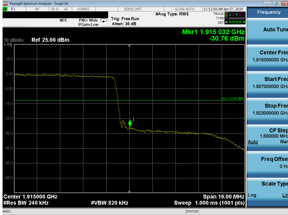
Plot 7-36. Upper Band Edge Plot (LTE Band 25 - 20MHz QPSK – Full RB Configuration)
