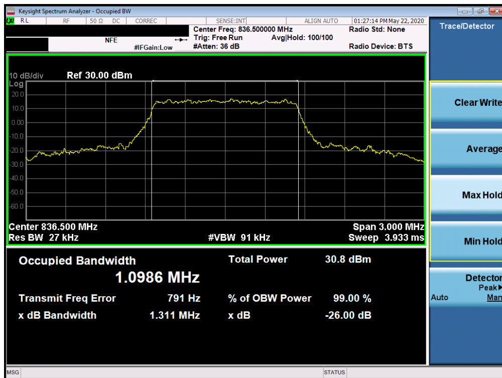
Plot 7-15. Occupied Bandwidth Plot (LTE Band 26/5 - 1.4MHz 64-QAM - Full RB Configuration)
