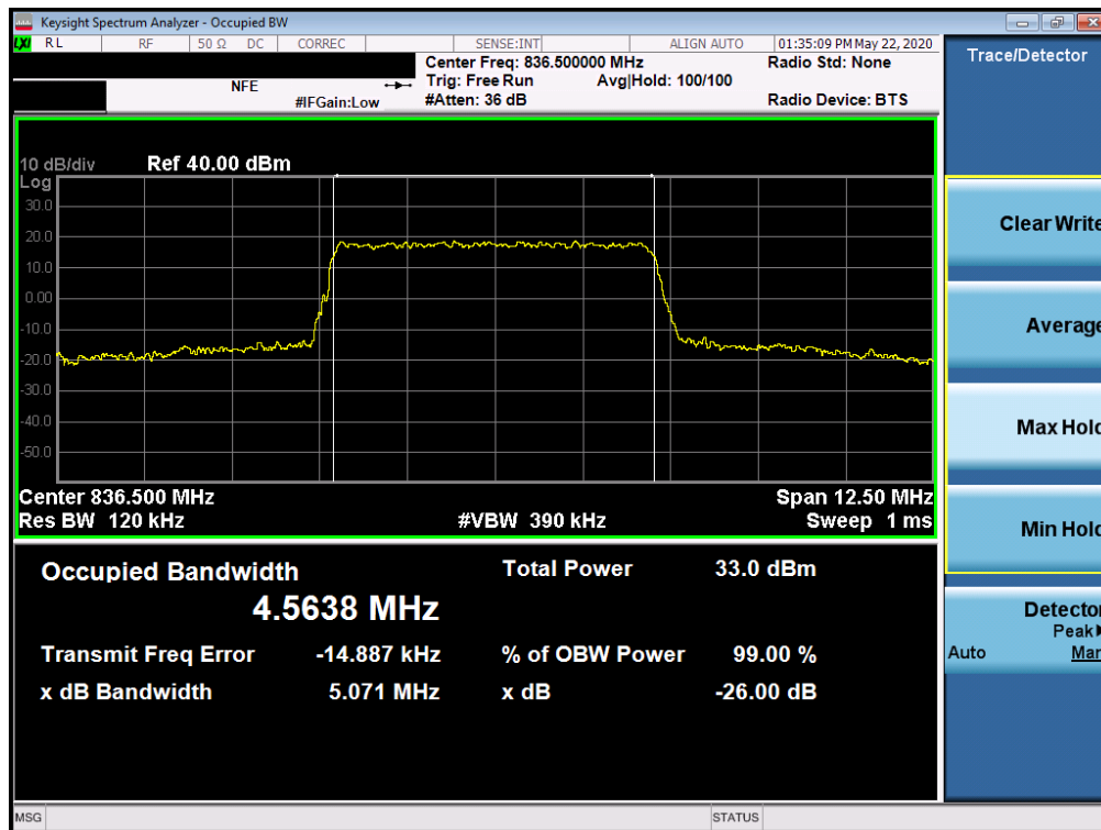
Plot 7-7. Occupied Bandwidth Plot (LTE Band 26/5 - 5MHz QPSK - Full RB Configuration)
