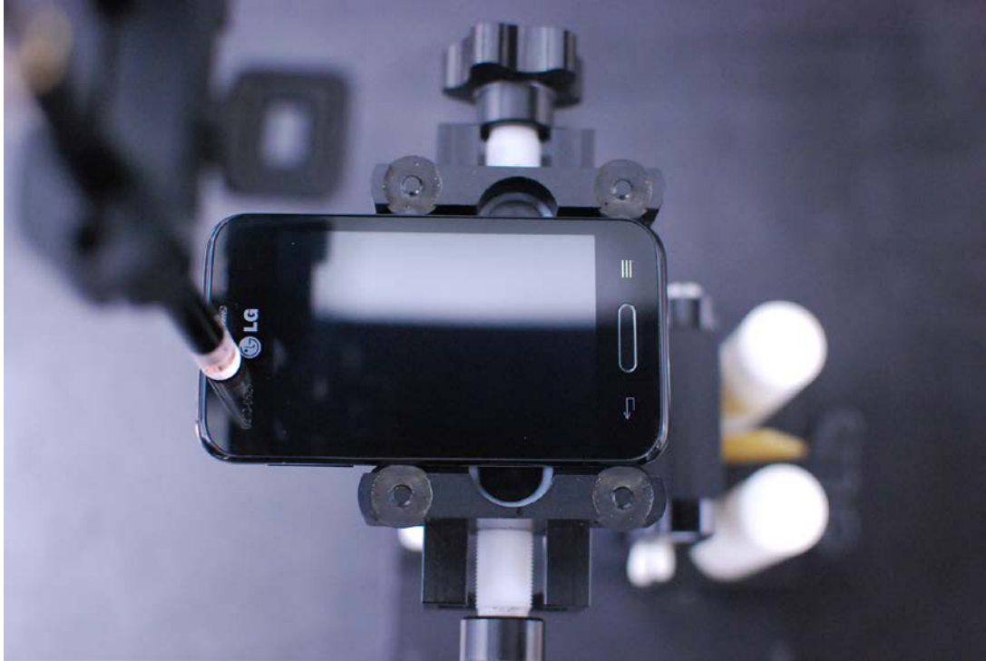
Figure 13-1 Test Setup for Wireless Device
