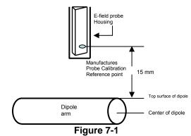
Separation Distance from Dipole to Field Probe
