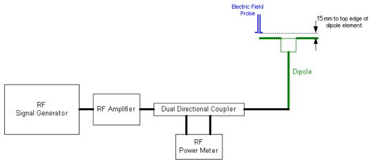
Figure 7-8 System Check Setup
