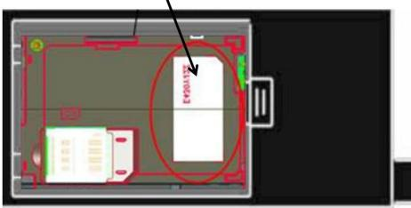
The label is placed inside of the battery compartment in back of the phone. When the user install the battery, the user can be the label.
