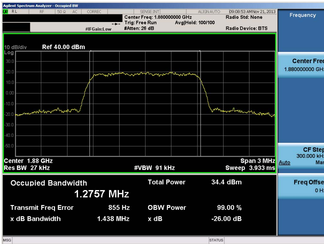
Plot 6-2. Occupied Bandwidth Plot (PCS CDMA Mode – Ch. 600)
