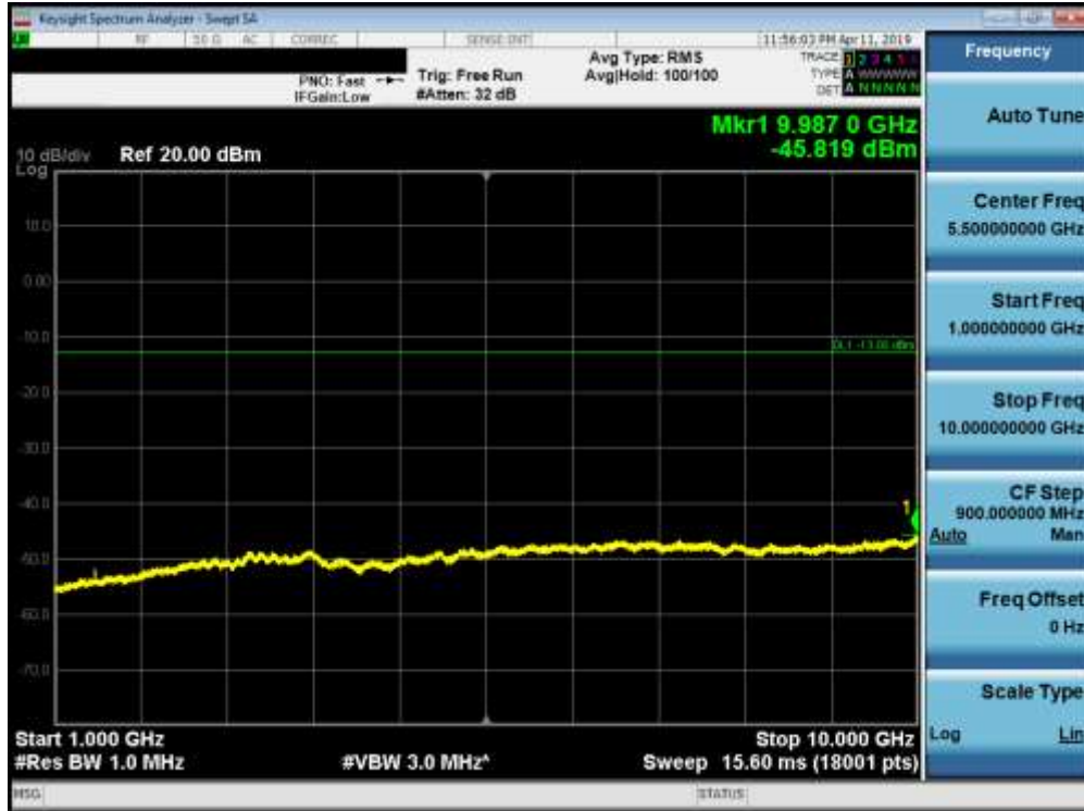
Plot 7-70. Conducted Spurious Plot (Band 12/17 - 10.0MHz QPSK - RB Size 1, RB Offset 0 - High Channel)
