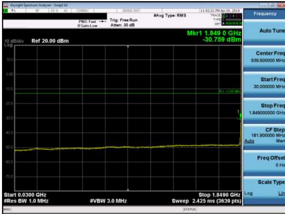
Plot 7-95. Conducted Spurious Plot (Band 2 - 20.0MHz QPSK - RB Size 1, RB Offset 0 - Low Channel)
