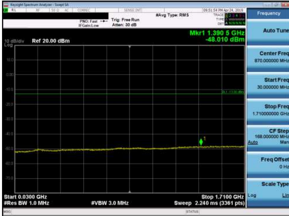
Plot 7-92. Conducted Spurious Plot (Band 66/4 - 20.0MHz QPSK - RB Size 1, RB Offset 0 - High Channel)
