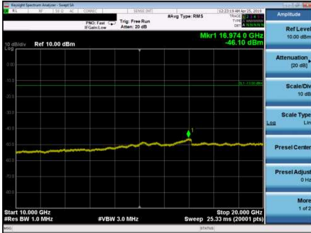
Plot 7-103. Conducted Spurious Plot (Band 2 - 20.0MHz QPSK - RB Size 1, RB Offset 0 - High Channel)
