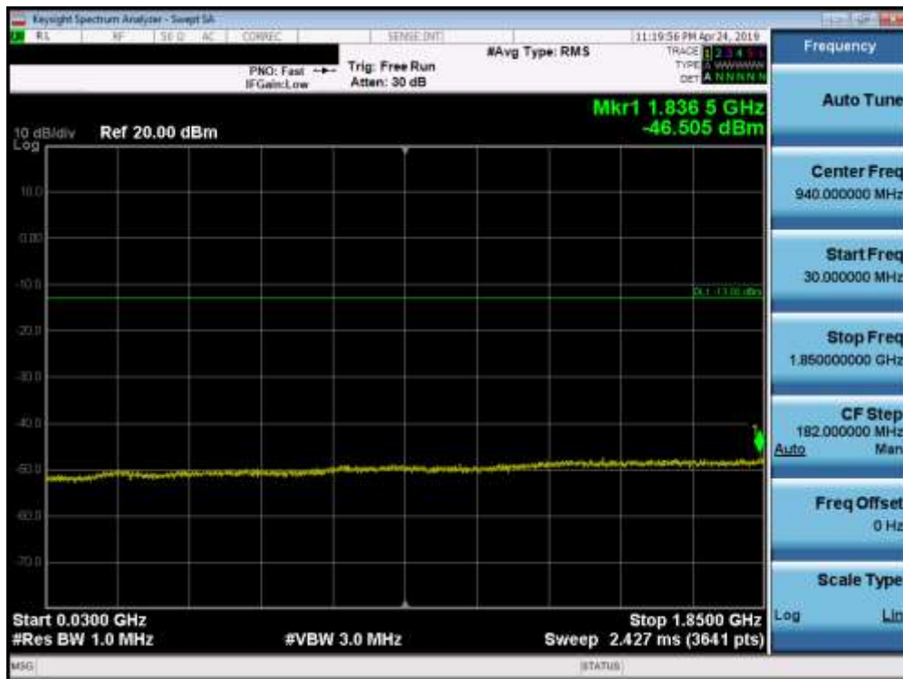
Plot 7-98. Conducted Spurious Plot (Band 2 - 20.0MHz QPSK - RB Size 1, RB Offset 0 - Mid Channel)
