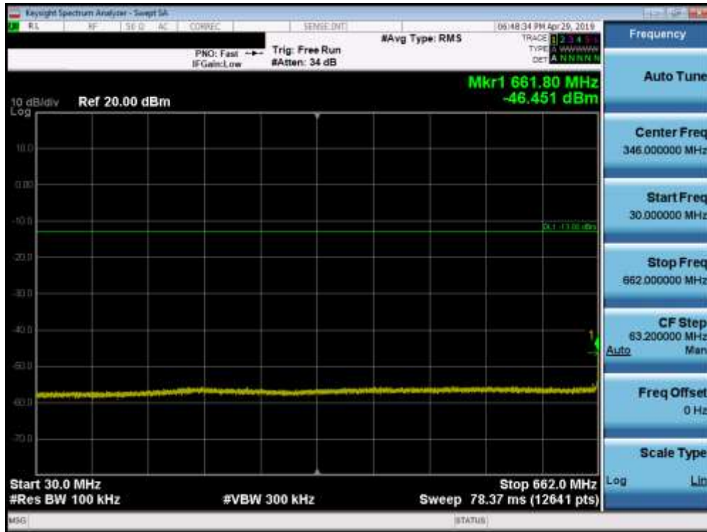
Plot 7-53. Conducted Spurious Plot (Band 71 - 20.0MHz QPSK - RB Size 1, RB Offset 0 - Low Channel)
