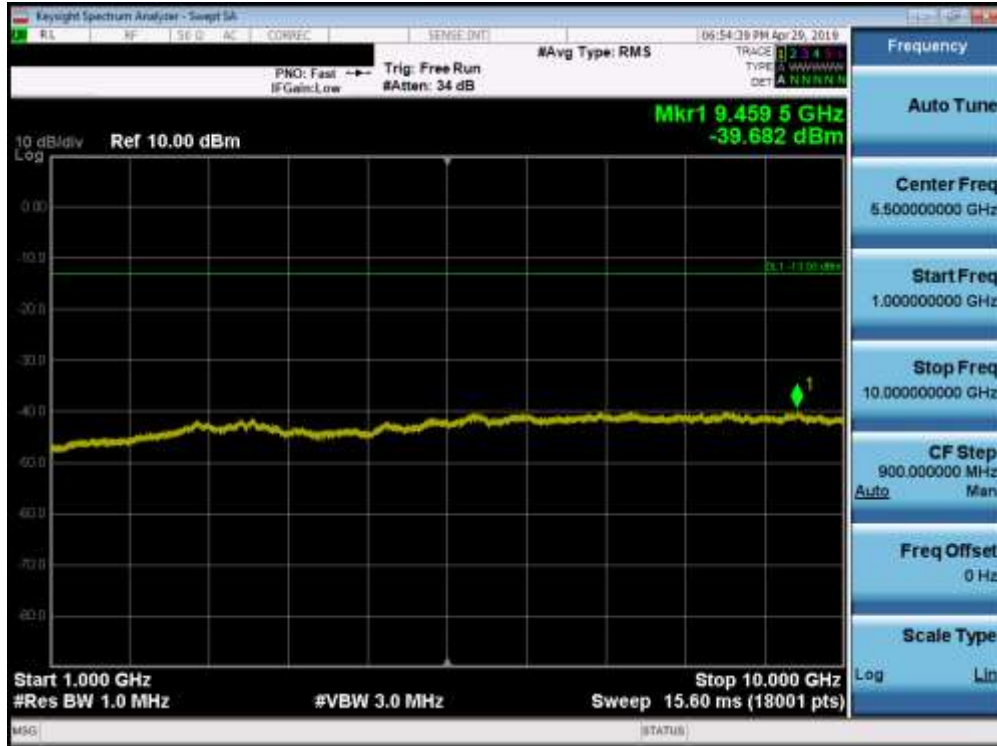
Plot 7-61. Conducted Spurious Plot (Band 71 - 20.0MHz QPSK - RB Size 1, RB Offset 0 - High Channel)
