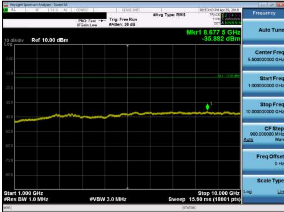
Plot 7-85. Conducted Spurious Plot (Band 5 - 10.0MHz QPSK - RB Size 1, RB Offset 0 - High Channel)
