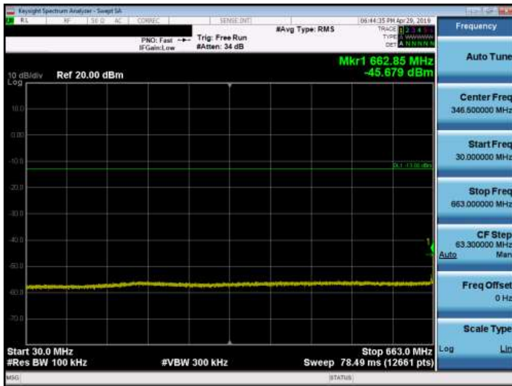
Plot 7-56. Conducted Spurious Plot (Band 71 - 20.0MHz QPSK - RB Size 1, RB Offset 0 - Mid Channel)
