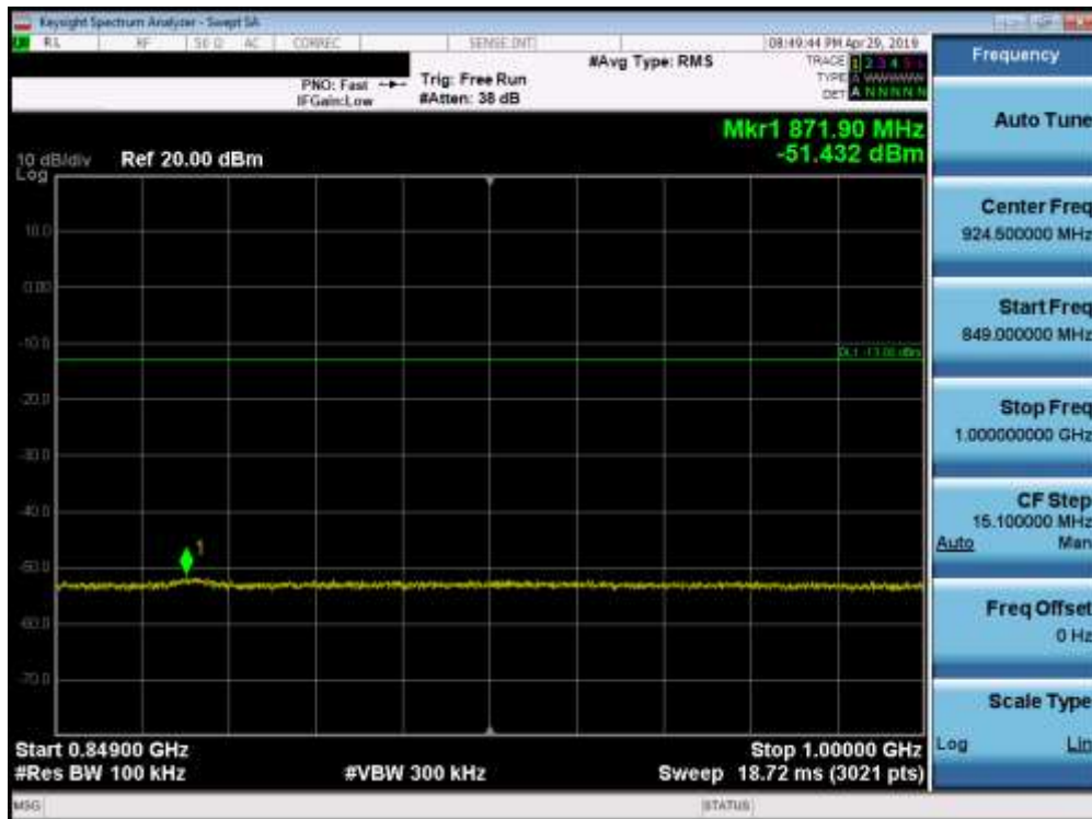
Plot 7-78. Conducted Spurious Plot (Band 5 - 10.0MHz QPSK - RB Size 1, RB Offset 0 - Low Channel)
