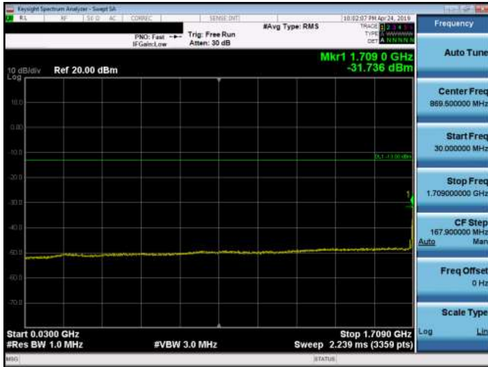
Plot 7-86. Conducted Spurious Plot (Band 66/4 - 20.0MHz QPSK - RB Size 1, RB Offset 0 - Low Channel)
