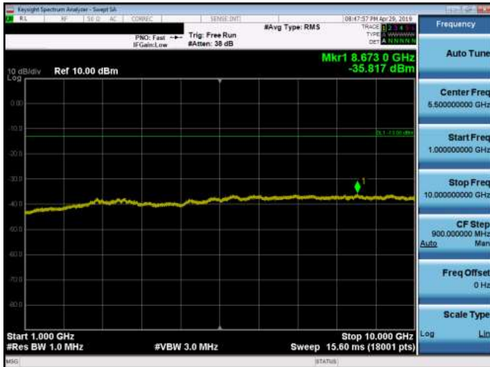
Plot 7-82. Conducted Spurious Plot (Band 5 - 10.0MHz QPSK - RB Size 1, RB Offset 0 - Mid Channel)
