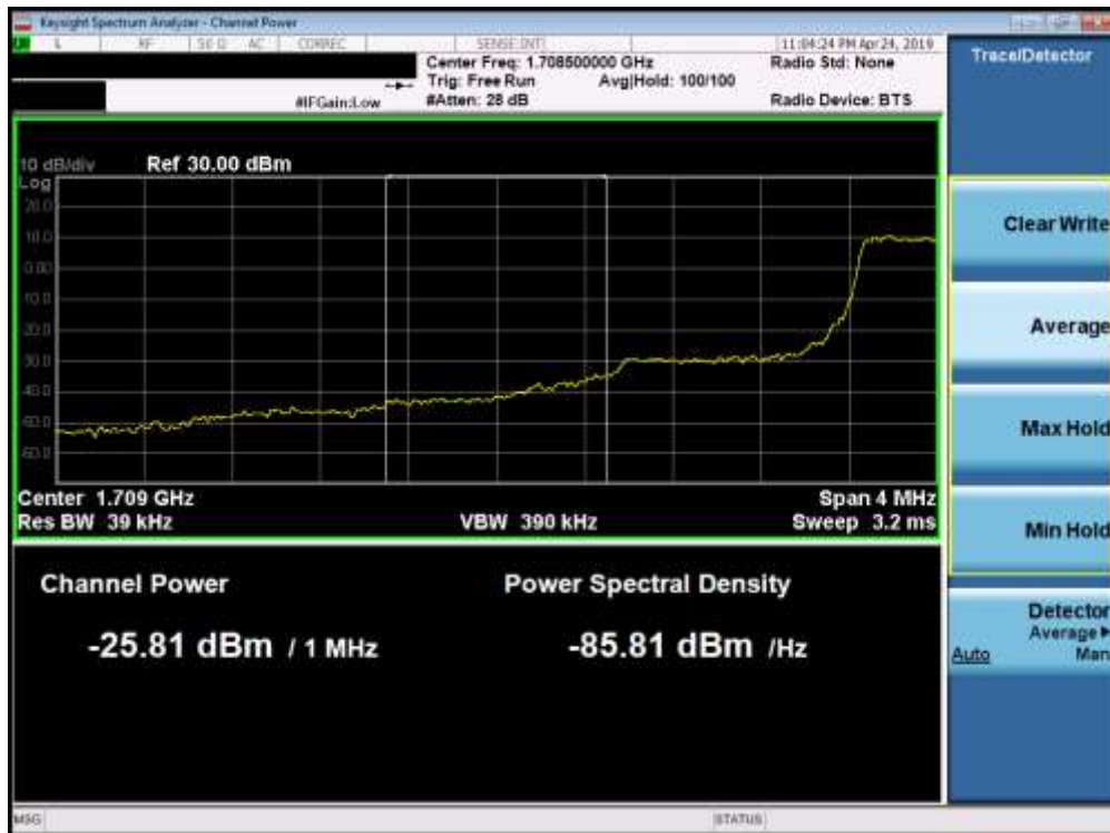
Plot 7-139. Lower Extended Band Edge Plot (Band 66/4 - 1.4MHz QPSK - Full RB Configuration)
