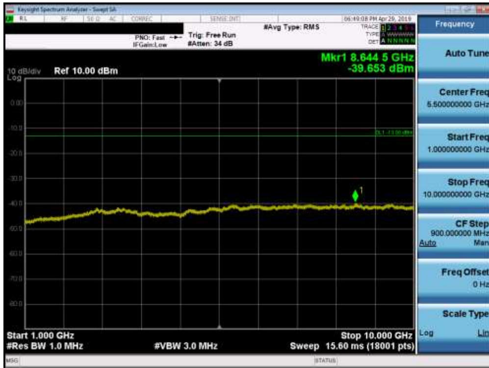
Plot 7-55. Conducted Spurious Plot (Band 71 - 20.0MHz QPSK - RB Size 1, RB Offset 0 - Low Channel)
