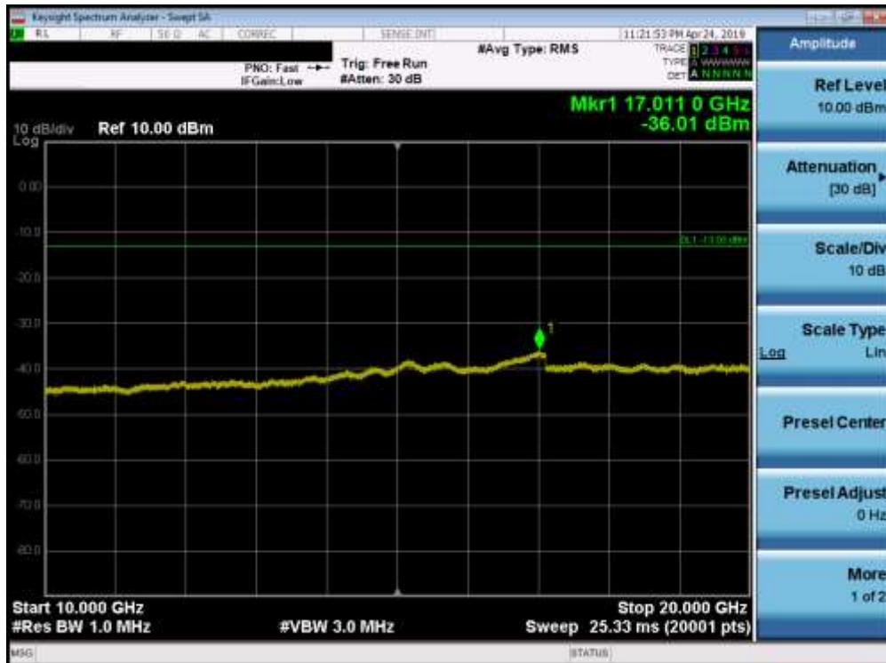
Plot 7-100. Conducted Spurious Plot (Band 2 - 20.0MHz QPSK - RB Size 1, RB Offset 0 - Mid Channel)
