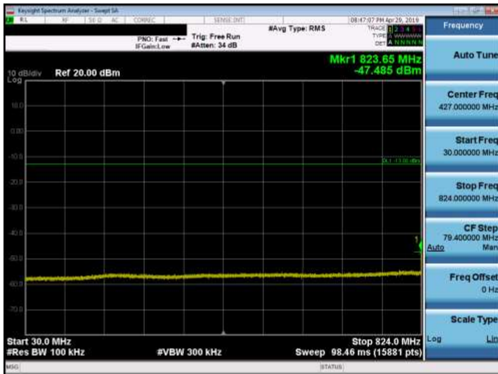
Plot 7-80. Conducted Spurious Plot (Band 5 - 10.0MHz QPSK - RB Size 1, RB Offset 0 - Mid Channel)
