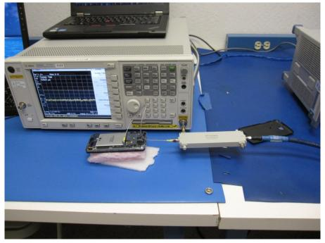
**RADIATED RF MEASUREMENT SETUP FOR PORTABLE CONFIGURATION**
