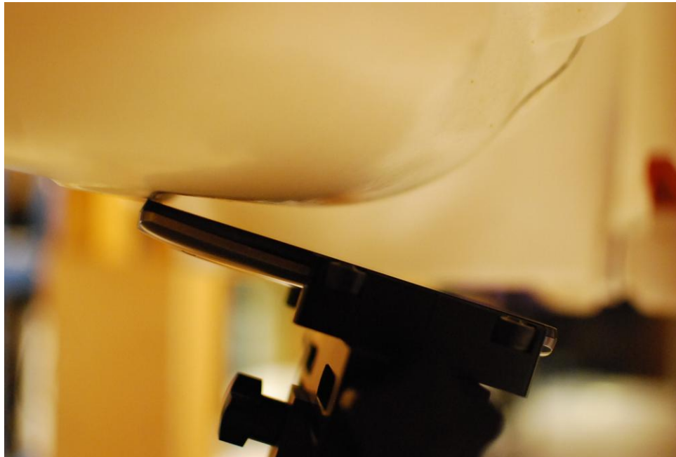
SAR Test Setup Photo 2: Right Tilt
