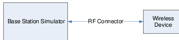
Figure 8-2 Power Measurement Setup
