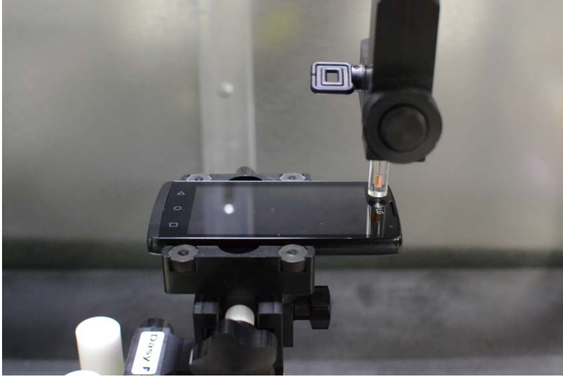
Figure 13-1 Test Setup for Wireless Device
