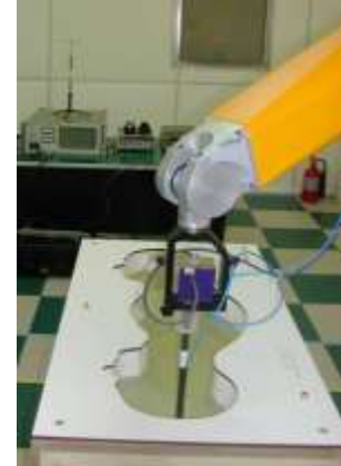
Figure 4.2 Photograph of the probe and the Phantom
