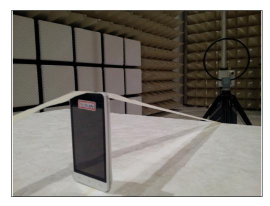
D. Photo of Field Strength & Spurious Emission Test for GSM
