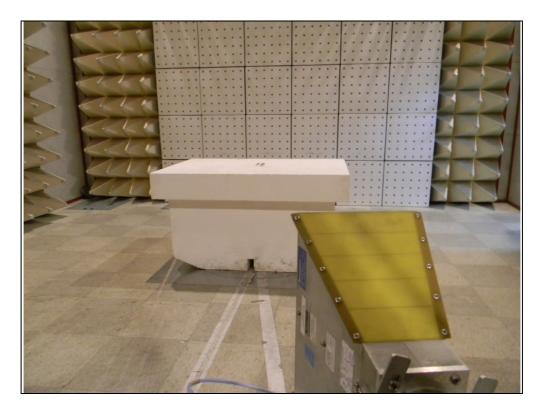
B. Photo of Field Strength & Spurious Emission Test for Bluetooth
