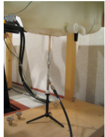
Photo of the dipole Antenna
