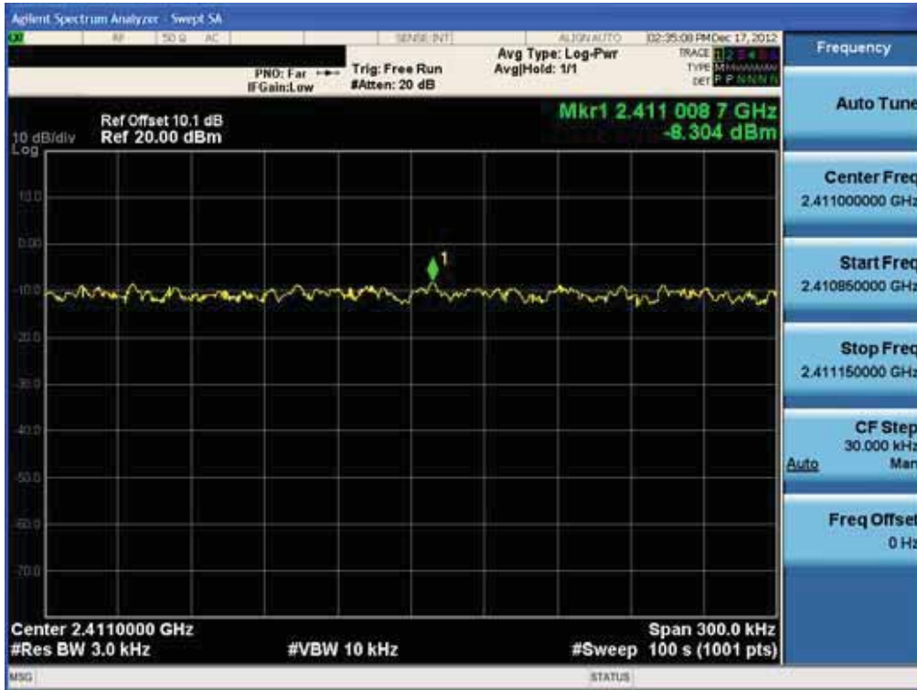
Power Spectral Density (802.11b-CH 6)
