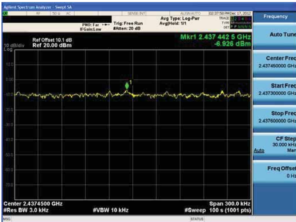
Power Spectral Density (802.11b-CH 6)
