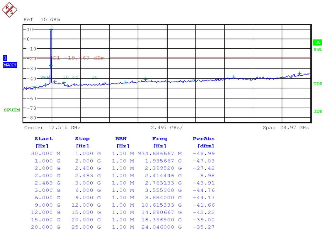
**Test Mode: Chain 1 & 802.11g & 6Mbps & 2437MHz****Reference**
