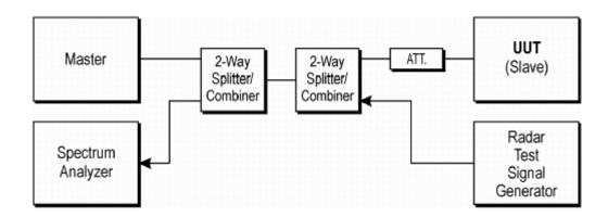
Figure 3-1. Conducted Test Setup for DFS
