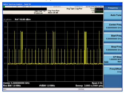
Time Display, WLAN Channel Traffic (Streaming Video)
