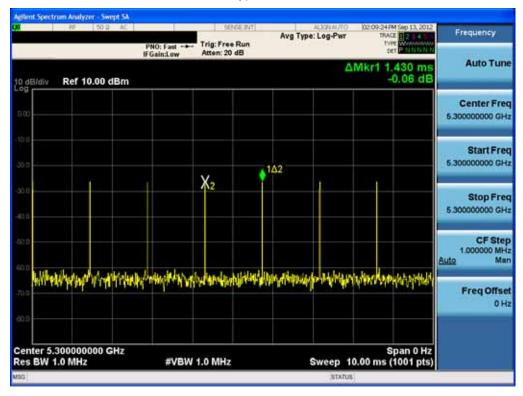
Time Display, Non WLAN Channel Traffic
