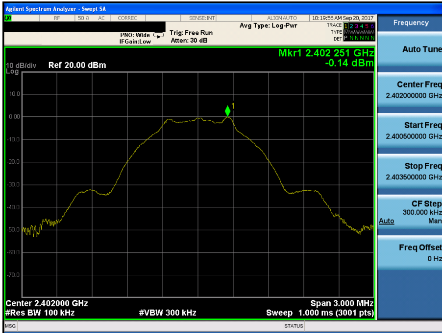
TM 1 Low Band-edge (Test Channel : Lowest)
